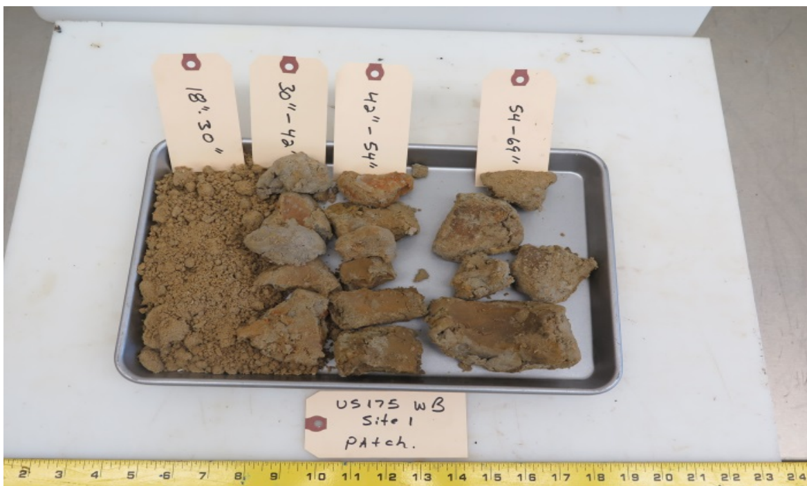
Figure 32. The Subgrade on Each Site Was Found to be a Tan Sandy Clay.
