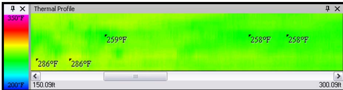
Figure 47. Moderate Thermal Segregation Barely Exceeding 25°F Threshold on Loop 340.
