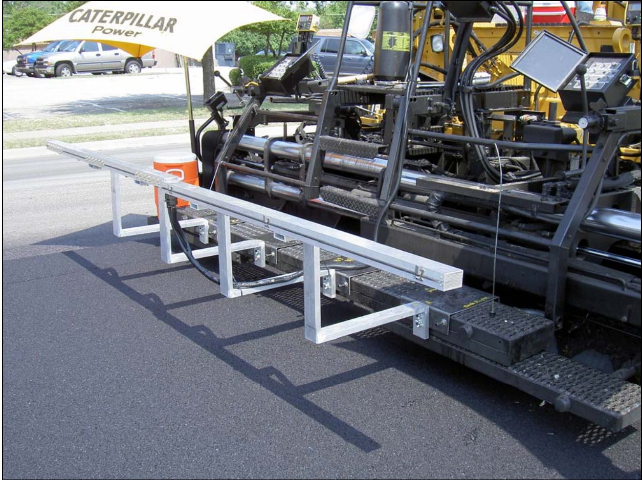
Figure 1.2. TTI's Current Pave-IR System Collecting Project Data.
