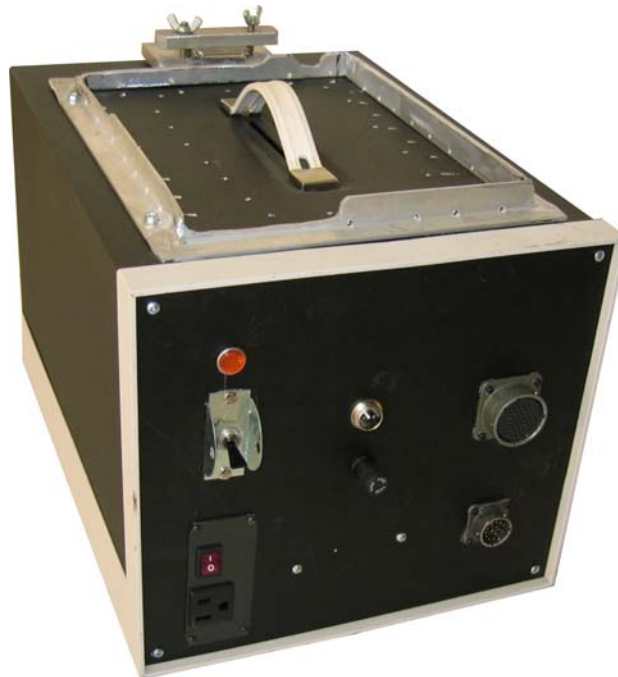
Figure 1.4. Master Control Box for Pave-IR.
