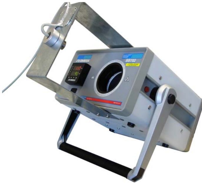
(a) Infrared Sensor in Blackbody for Calibration.
