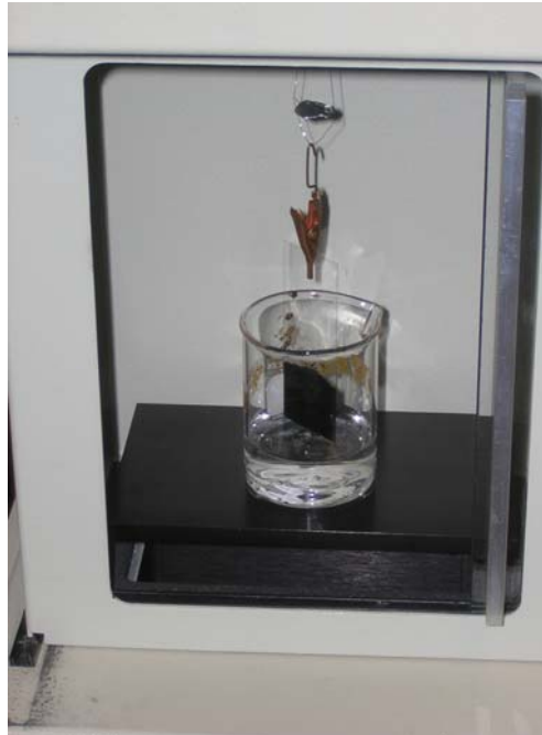
Figure C.3. Asphalt Binder Sample Suspended from Micro Balance for Immersion in Probe Liquid.
