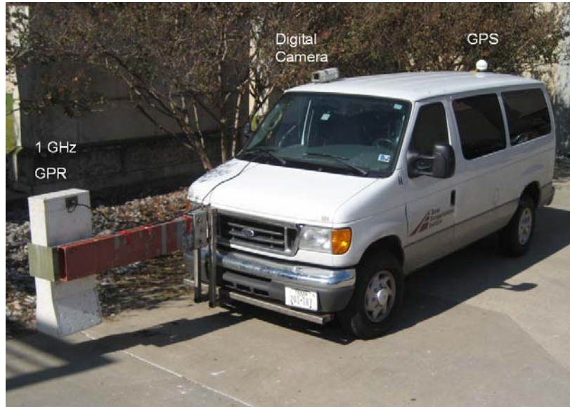
Figure 2. TTI's Latest GPR Vehicle with GPS.
