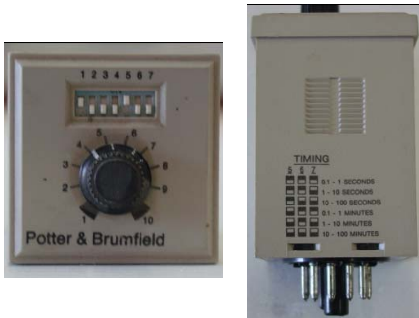
Figure 27. Time Delay Flasher Control Relay.
