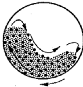
Figure 2.6. Schematic of Interaction between Aggregates and Steel Balls in Presence of Water in the Micro-Deval.
