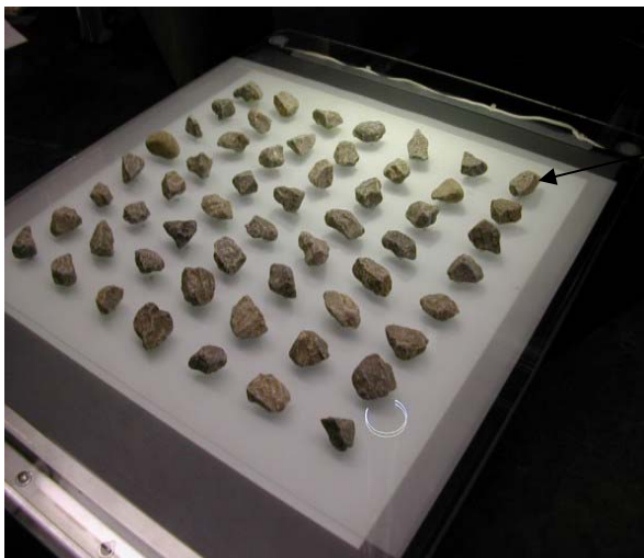
Figure 13. Coarse Aggregates Properly Positioned on Glass Tray.
