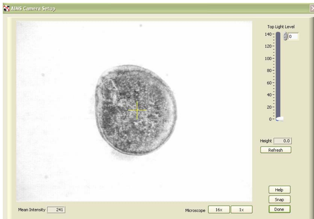
Figure 7. Calibration Point Centered at an Intermediate Magnification.
