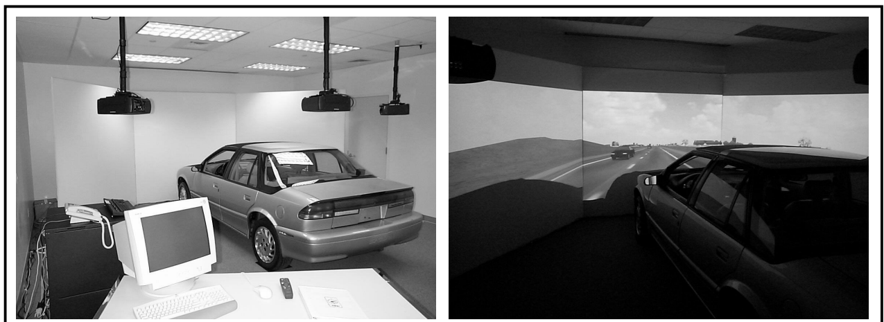
Figure 21. Photos of the Driving Environment Simulator at Texas A&M University.
