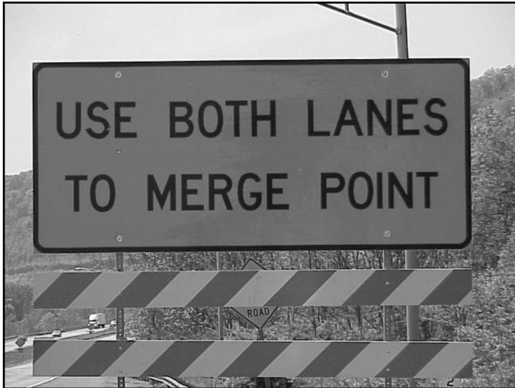
Figure 12. 'Use Both Lanes to Merge Point' Sign Used in Pennsylvania.
