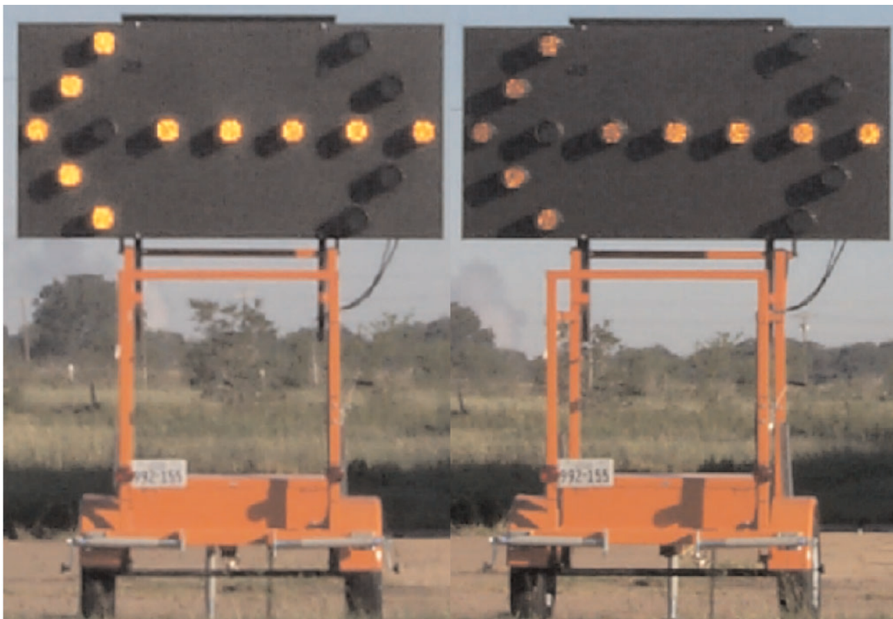
Figure 3. The effect of angularity on arrow panel visibility (the arrow sign on the right is at a slight angle)
