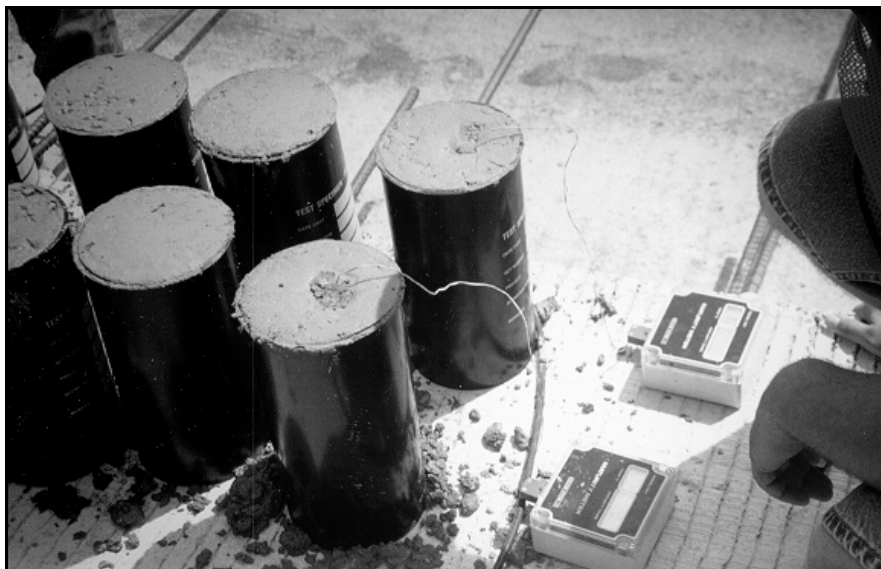
Figure 3.19 Maturity of Concrete Cylinders Was Monitored at the Test Site.
