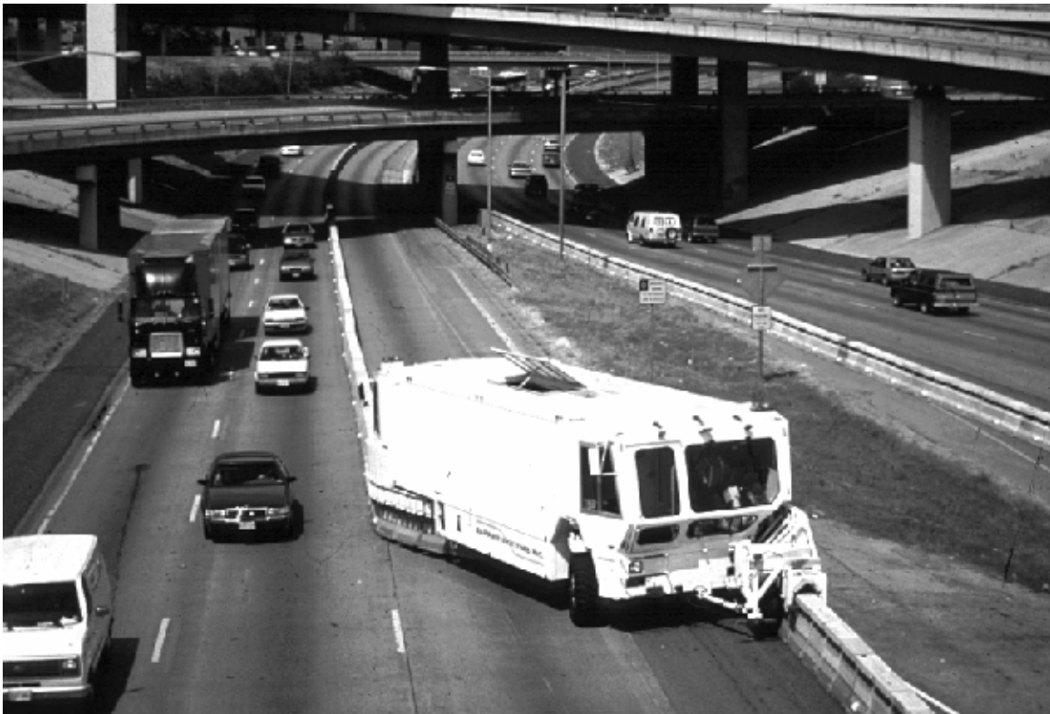
Figure 8. IH-30 East R. L. Thornton Freeway Moveable-Barrier Contraflow HOV Lane in Dallas, Texas (2).
