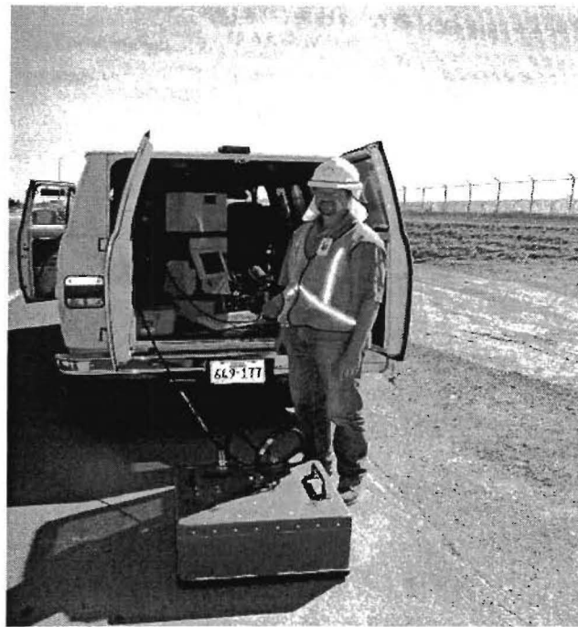
Figure 3. Data Collection with a 200 MHz Ground-Coupled System.
