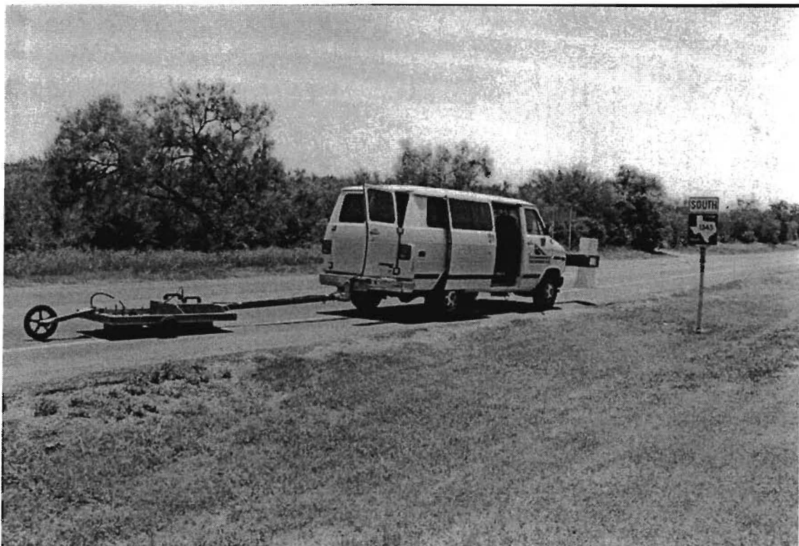
Figure 4. Simultaneously Collecting Air-Launched and Ground-Coupled GPR Data.
