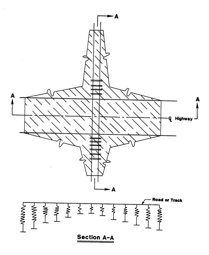
Figure 7. Variable Stiffness of Road and Track
