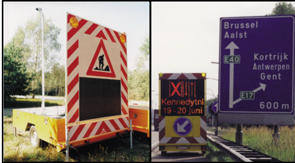
Figure 2-8. Trailer-Mounted VMS for Queue Detection and Warning. 27
