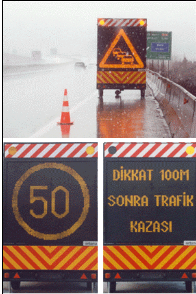
Figure 2-31. Mobile Variable Message Sign Trailers on Turkish Motorways. 47
