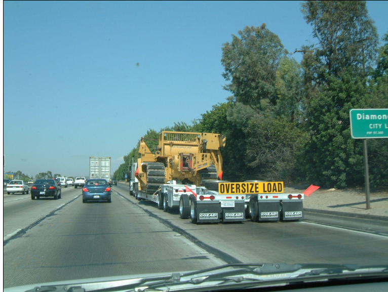
Figure 16. Oversize Load on 12-ft Lane.
