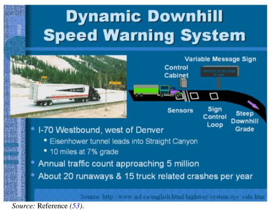
Figure 18. Downhill Speed Warning System.
