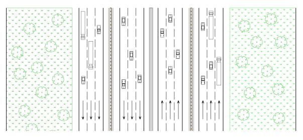
Figure 10. Typical Cross-Section of Dual-Dual Roadway.
