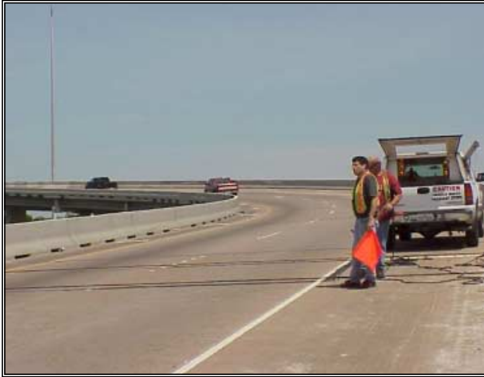
Figure 9. Field Installation of Road Tubes for Classification Studies.
