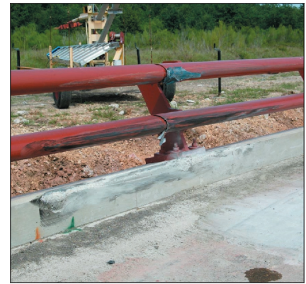
Damage to Texas T77 after small car test.
