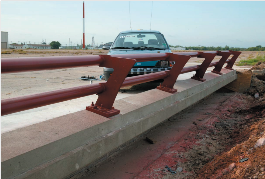
Texas T77 bridge railing with small car.
