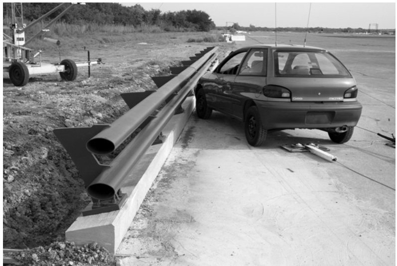
Figure 27. Vehicle/Bridge Rail Geometrics for Test 442882-4.
