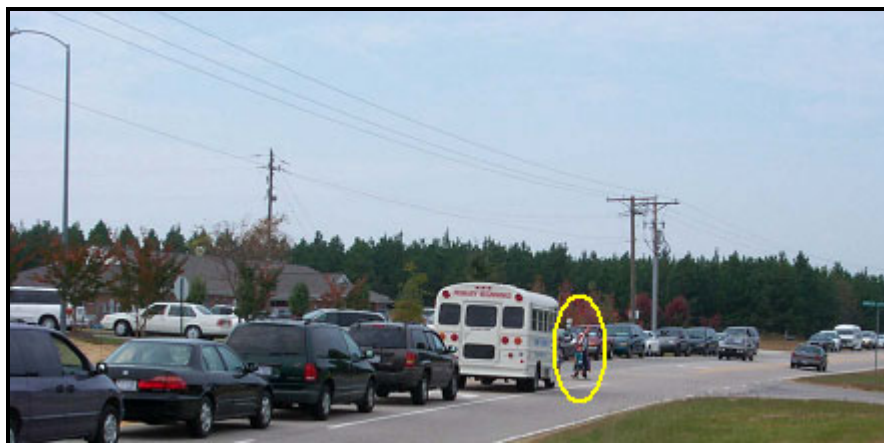
Figure 32. Jaywalking across Street Adjacent to the School Site – No Marked Crosswalk.
