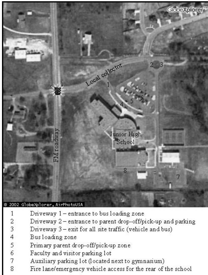
Figure 7-180. Middle School Case Study Site 5 Aerial Photograph (Base Aerial Photograph Is from GlobeXplorer (45)).
