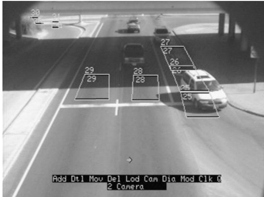
Figure 12. Shadows from Tall Vehicles and Bridge Structures.
