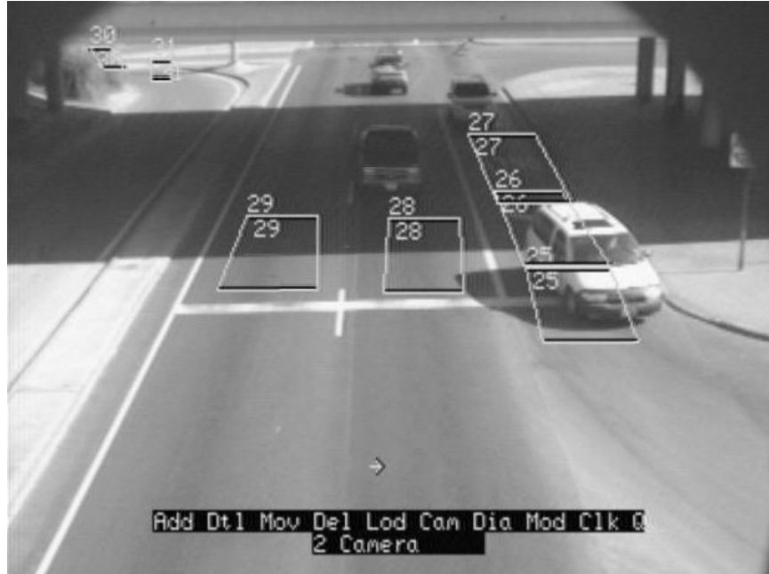
Figure 3-2. Shadows from Tall Vehicles and Bridge Structures.
