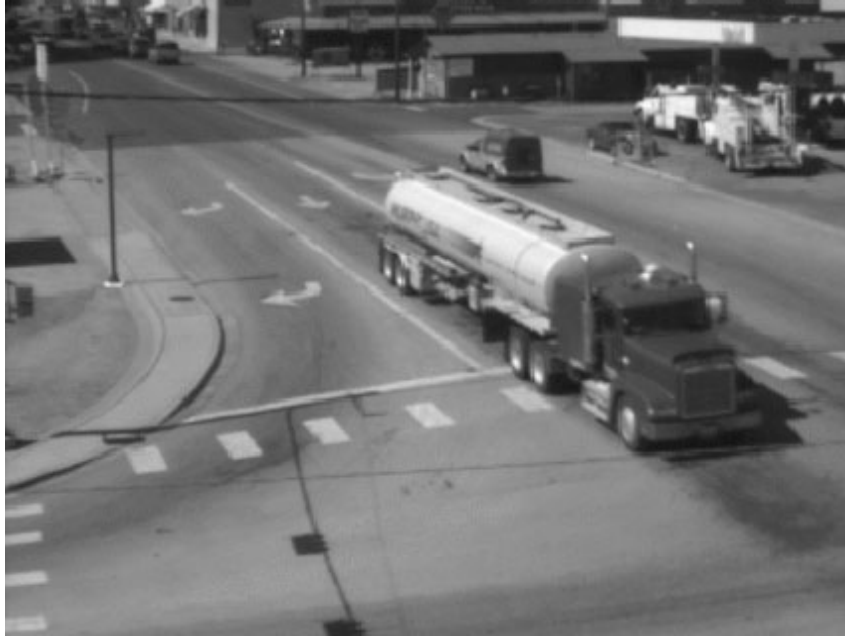
Figure 2-5. Adjacent-Lane Occlusion with Right-Side Camera.
