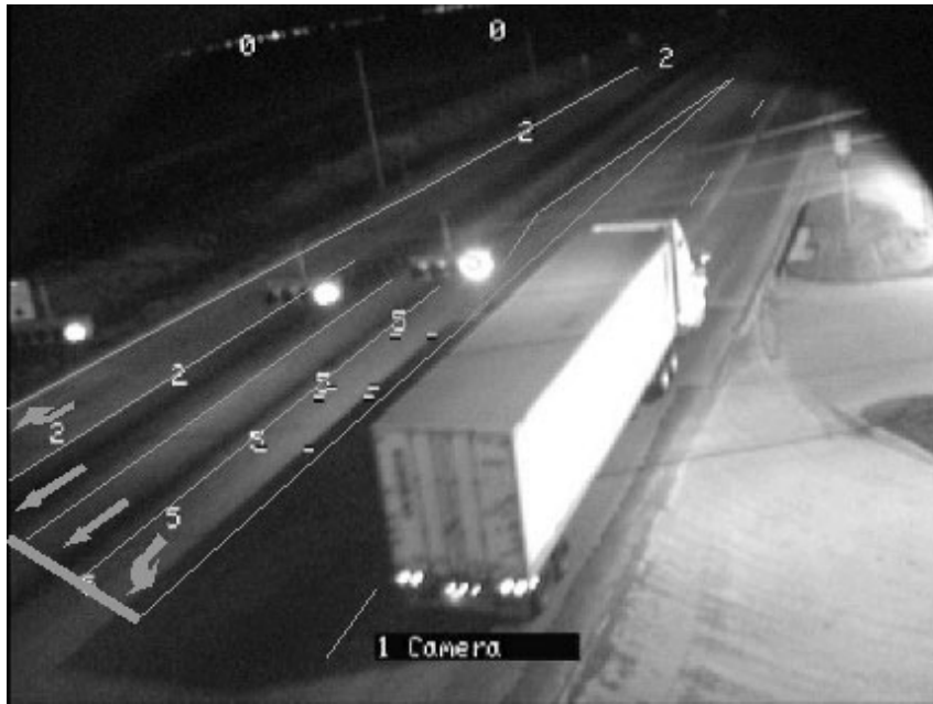
Figure 2-6. Adjacent-Lane Occlusion with Left-Side Camera.
