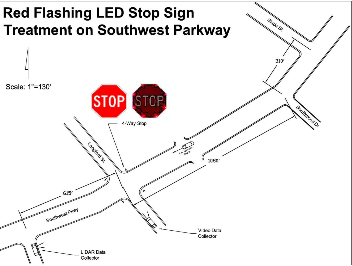
Figure A-13. Plan View of Southwest Parkway @ Langford St. in College Station, Texas.
