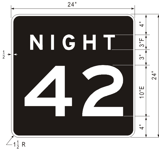
Figure 8. Design of Nighttime Speed Limit (R2-3) Signs.
