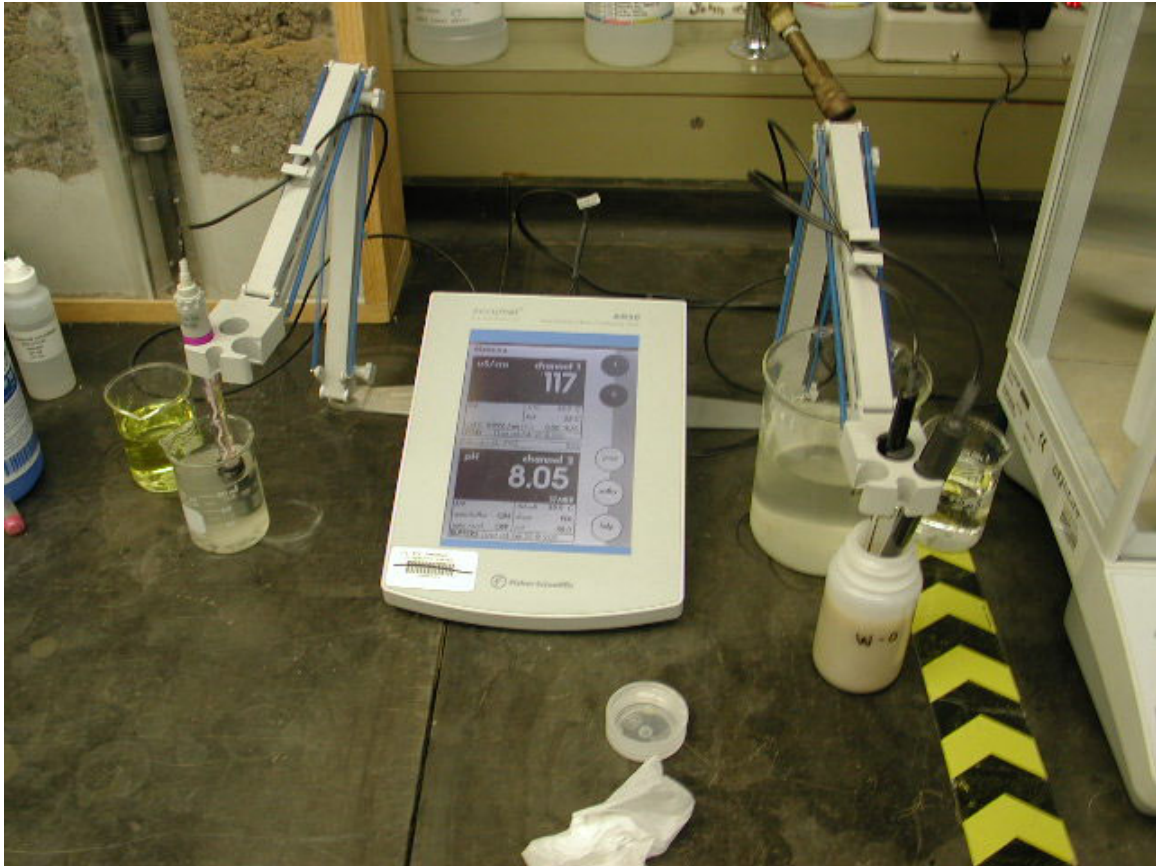
Figure 7. Accumet Model AR50 pH/Conductivity Meter.
