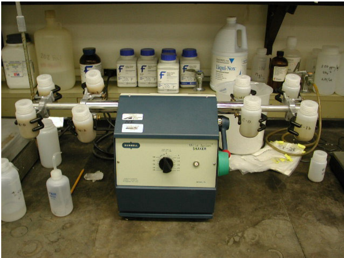
Figure 8. Burrell Model 75 Shaker for Conductivity Measurements. Note: The 125 ml Nalgene Bottles Attached to the Shaker.
