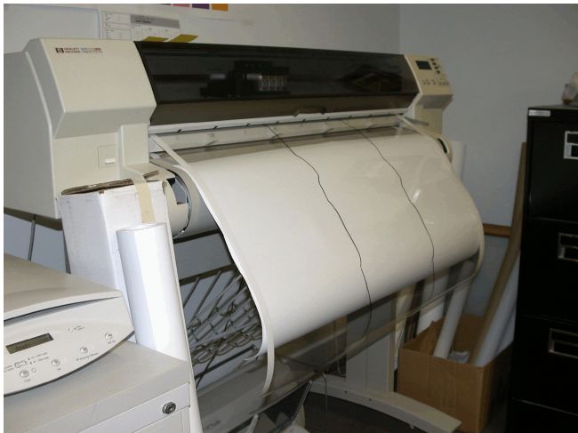
Figure 5. Printing Simulated Crack.
