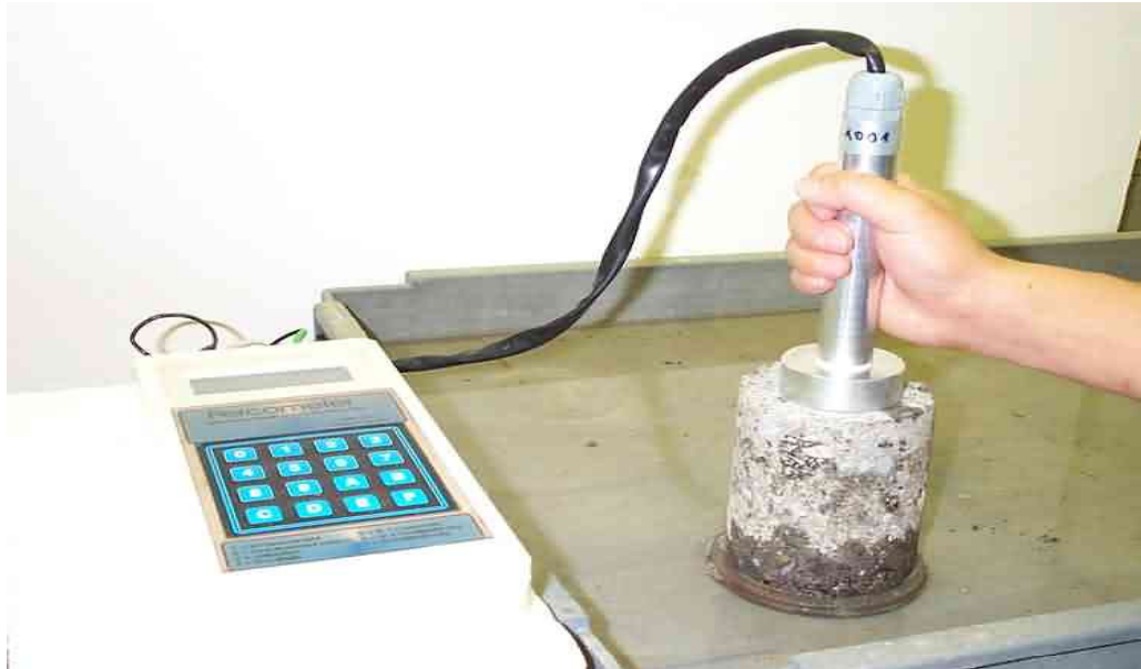
Figure 47. Dielectric Constant Value Measurement Using the Adek Probe.
