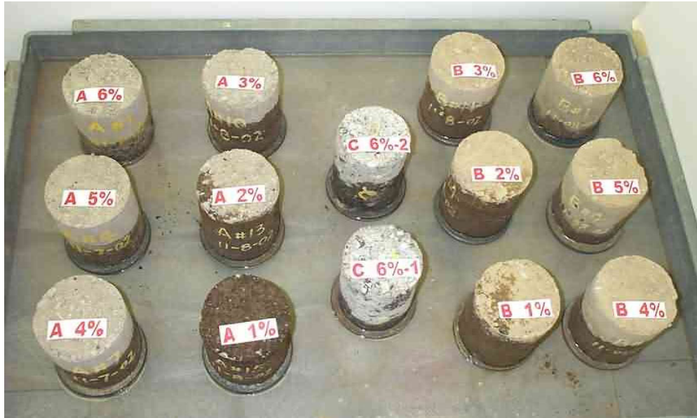
Figure 46. TST Setup for Stabilized Base Idaho Samples.
