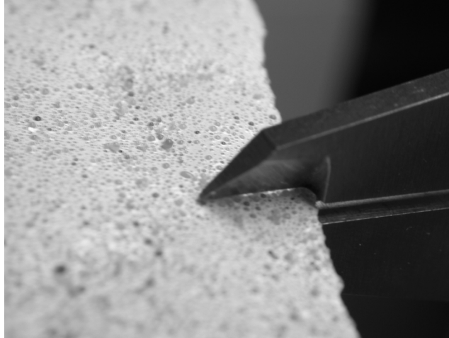
Figure 4. Top-of-Bead Measurement with Caliper.
