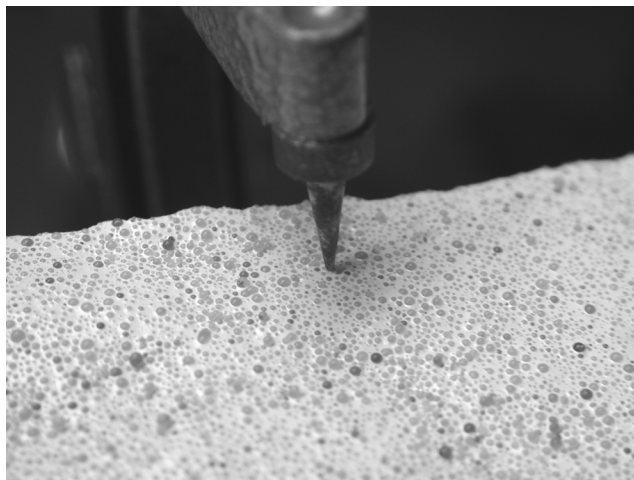
Figure 3. Binder-Only Measurement with Needlepoint Micrometer.
