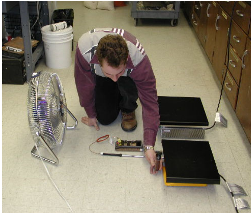
Figure 19. Setup and Wind Speed Being Measured for Lab Testing with Wind.
