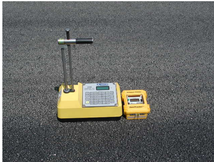
Figure F1. Nuclear Gauge (left) vs. Pavetracker (right).
