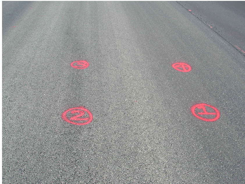
Figure 59. Locations of Cores 1-4 on IH 10 Test Section.
