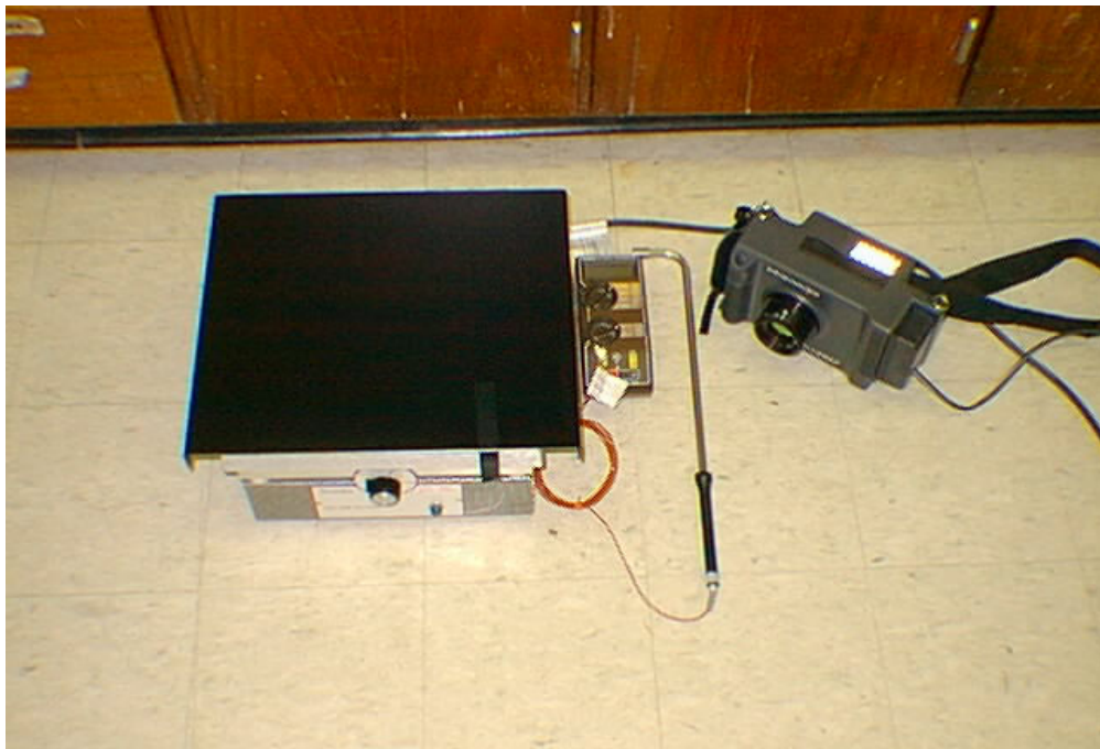
Figure 7. Equipment for Lab Verification of Infrared Equipment.
