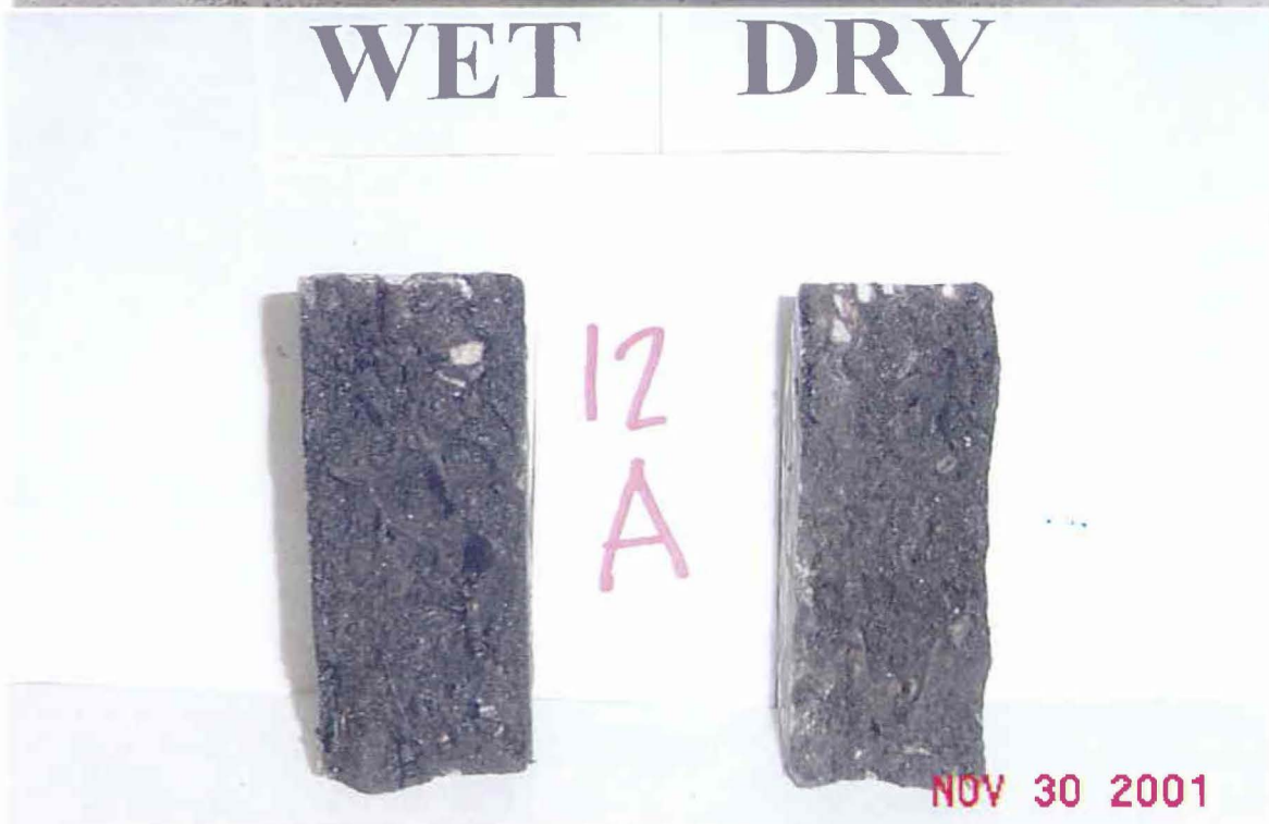
Figure B8. Photographs of the Cores after Hamburg and TSR Tests (Atlanta – Section 8 – IH 30).
