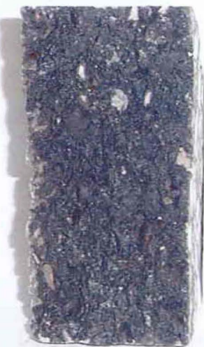
Figure B5. Photographs of the Cores after Hamburg and TSR Tests (Atlanta – Section 5 – FM 881).
