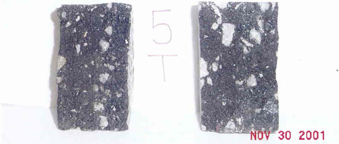
Figure B29. Photographs of the Cores after Hamburg and TSR Tests (Tyler – Section 5 – SH 31).
