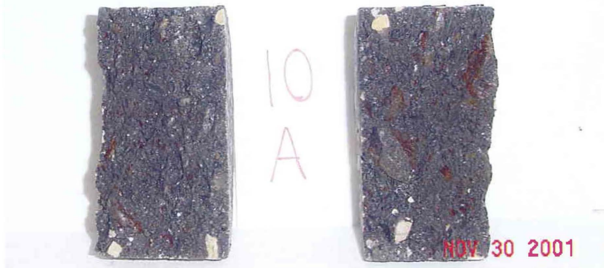
Figure B6. Photographs of the Cores after Hamburg and TSR Tests (Atlanta – Section 6 – US 59).
