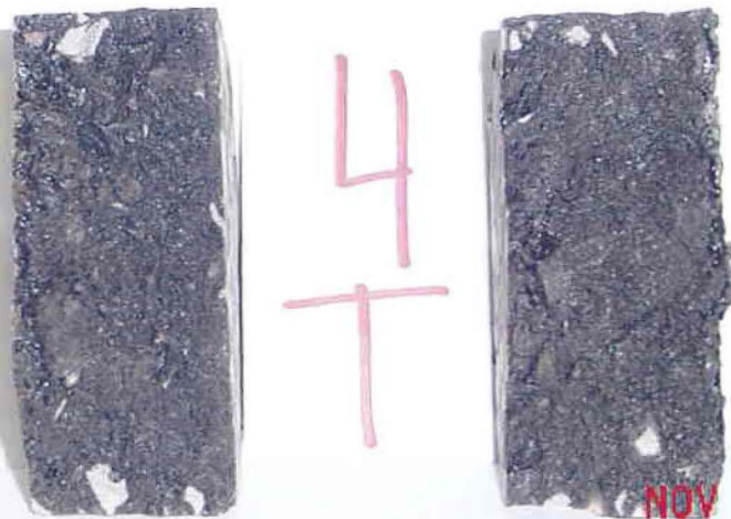
Figure C28. Photographs of the Cores after Hamburg and TSR Tests (Tyler - Section 4 - US 69).
