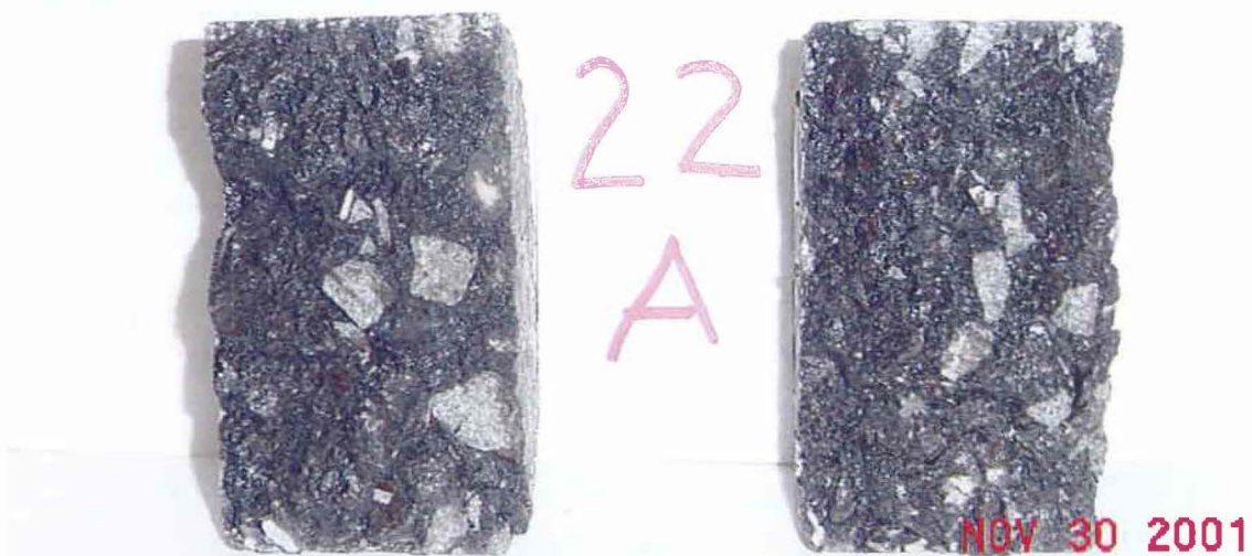
Figure B11. Photographs of the Cores after Hamburg and TSR Tests (Atlanta - Section 11 - US 79).
