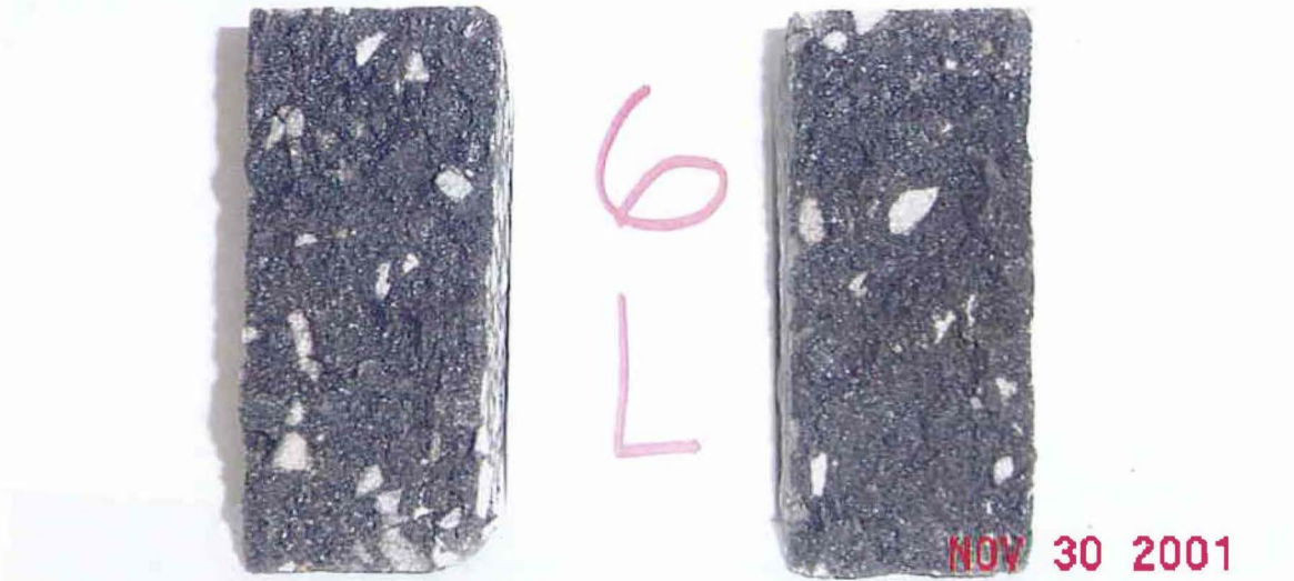
Figure B23. Photographs of the Cores after Hamburg and TSR Tests (Lufkin – Section 6 – US 59).
