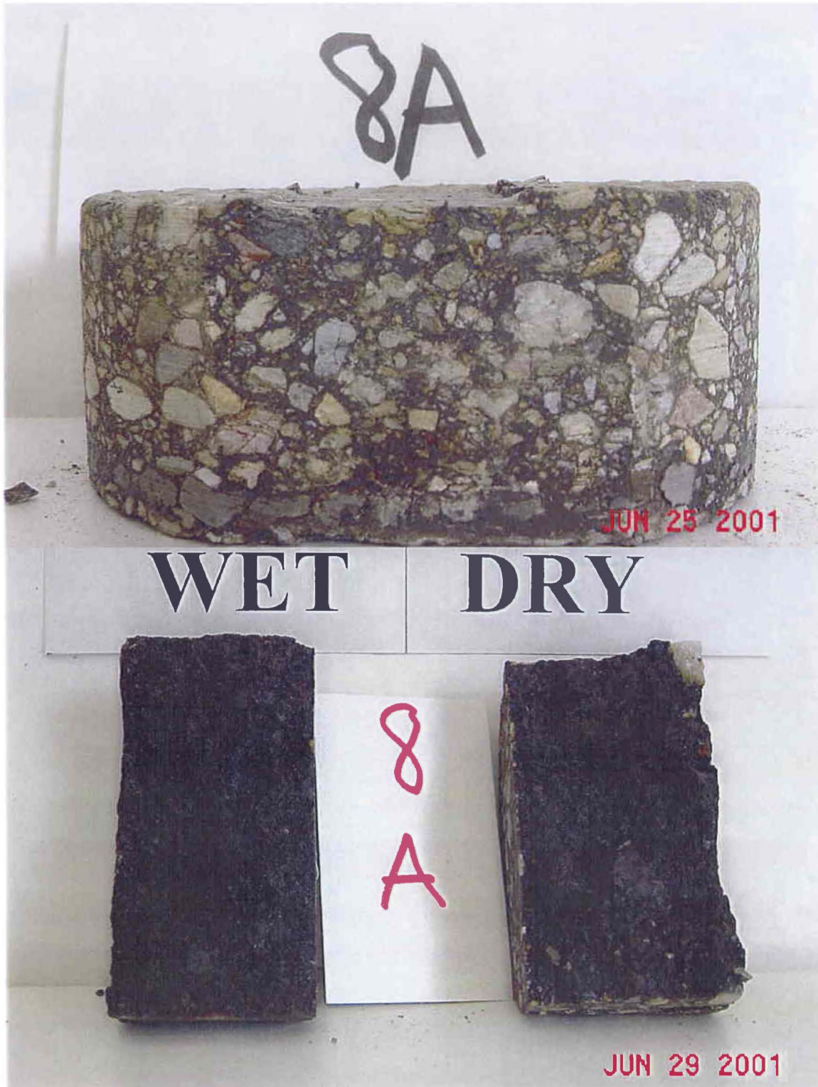
Figure B4. Photographs of the Cores after Hamburg and TSR Tests (Atlanta – Section 4 – IH 30).
