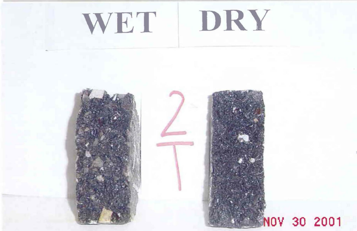
Figure B26. Photographs of the Cores after Hamburg and TSR Tests (Tyler – Section 2 – US 69).
