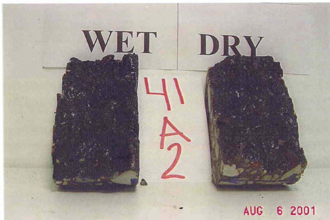
Figure B18. Photographs of the Cores after Hamburg and TSR Tests (Atlanta – Section 18(2) – US 59).
