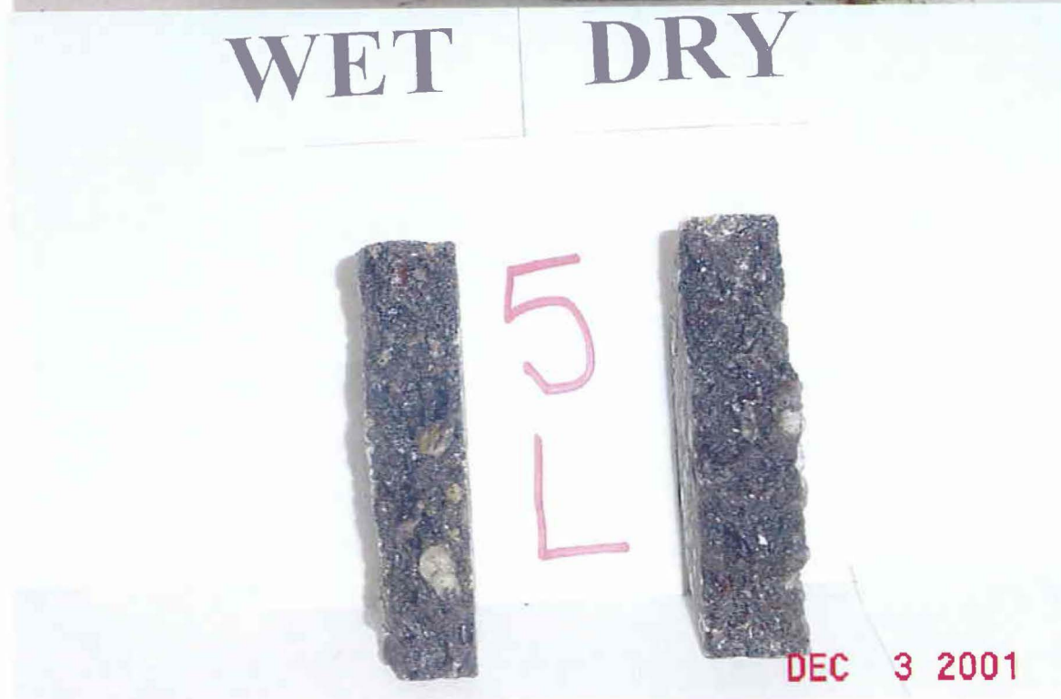
Figure B22. Photographs of the Cores after Hamburg and TSR Tests (Lufkin - Section 5 - US 59).
