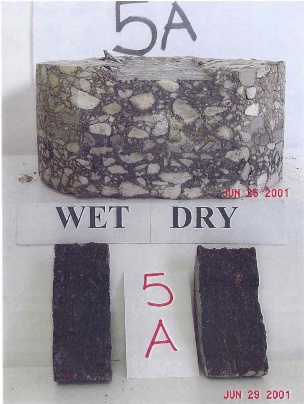
Figure B2. Photographs of the Cores after Hamburg and TSR Tests (Atlanta – Section 2 – US 67).
