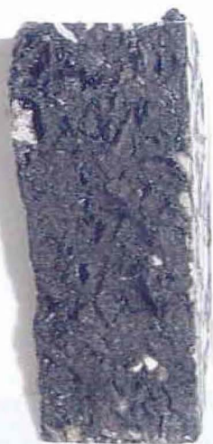
Figure B15. Photographs of the Cores after Hamburg and TSR Tests (Atlanta – Section 15 – US 271).
