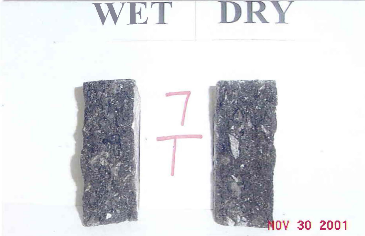
Figure B31. Photographs of the Cores after Hamburg and TSR Tests (Tyler - Section 7 - IH 20).
