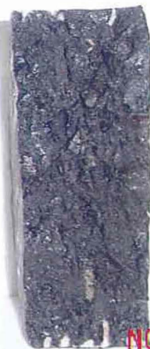
Figure B15. Photographs of the Cores after Hamburg and TSR Tests (Atlanta – Section 15 – US 271).
