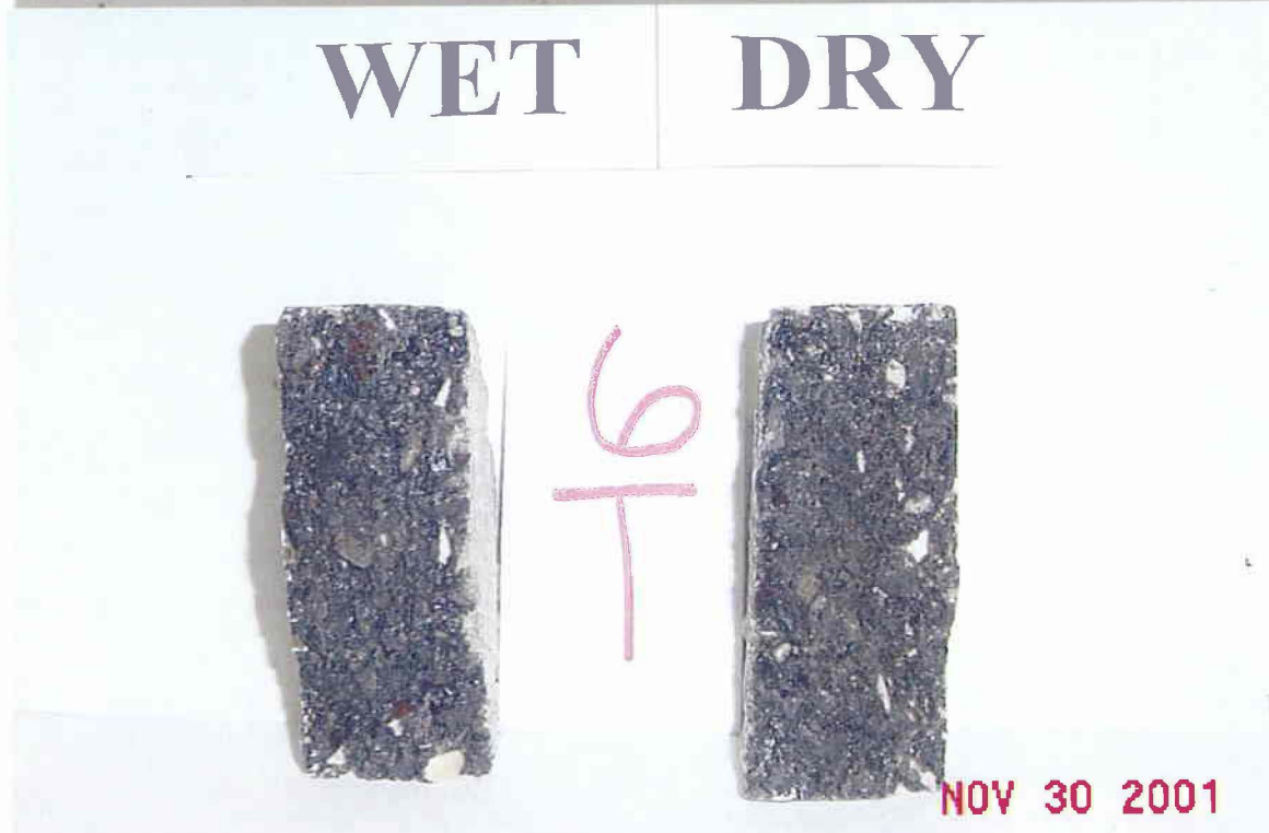
Figure B30. Photographs of the Cores after Hamburg and TSR Tests (Tyler - Section 6 - US 79).
