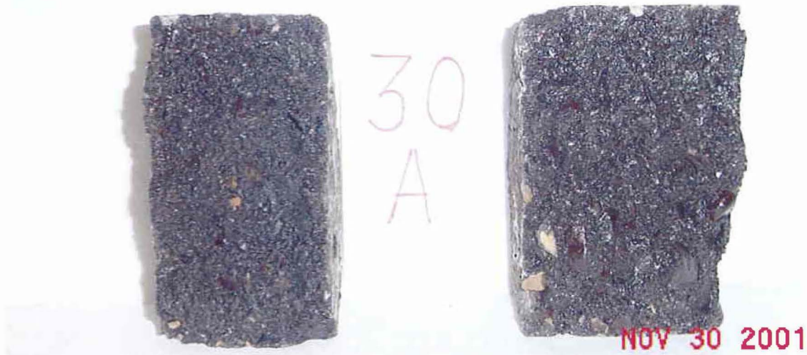
Figure B14. Photographs of the Cores after Hamburg and TSR Tests (Atlanta – Section 14 – SH 43).
