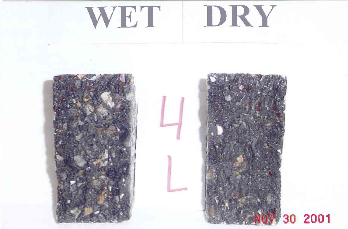
Figure B21. Photographs of the Cores after Hamburg and TSR Tests (Lufkin – Section 4 – US 259).
