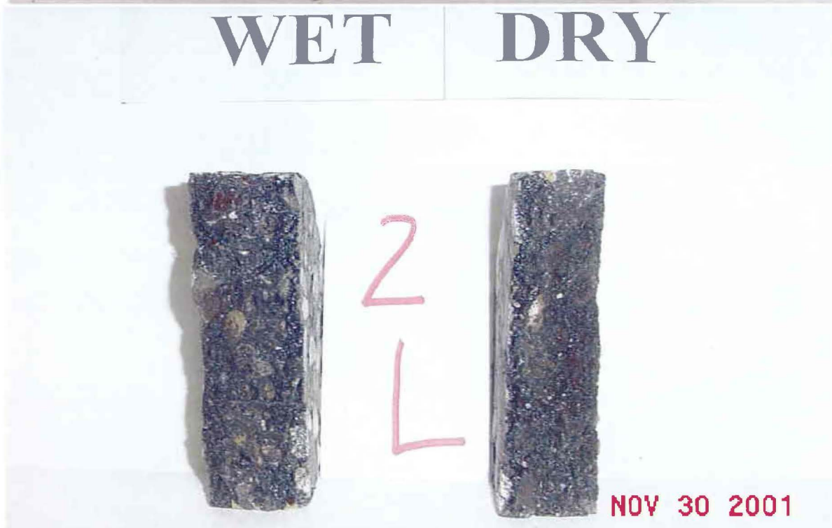
Figure B19. Photographs of the Cores after Hamburg and TSR Tests (Lufkin – Section 2 – SH 7).
