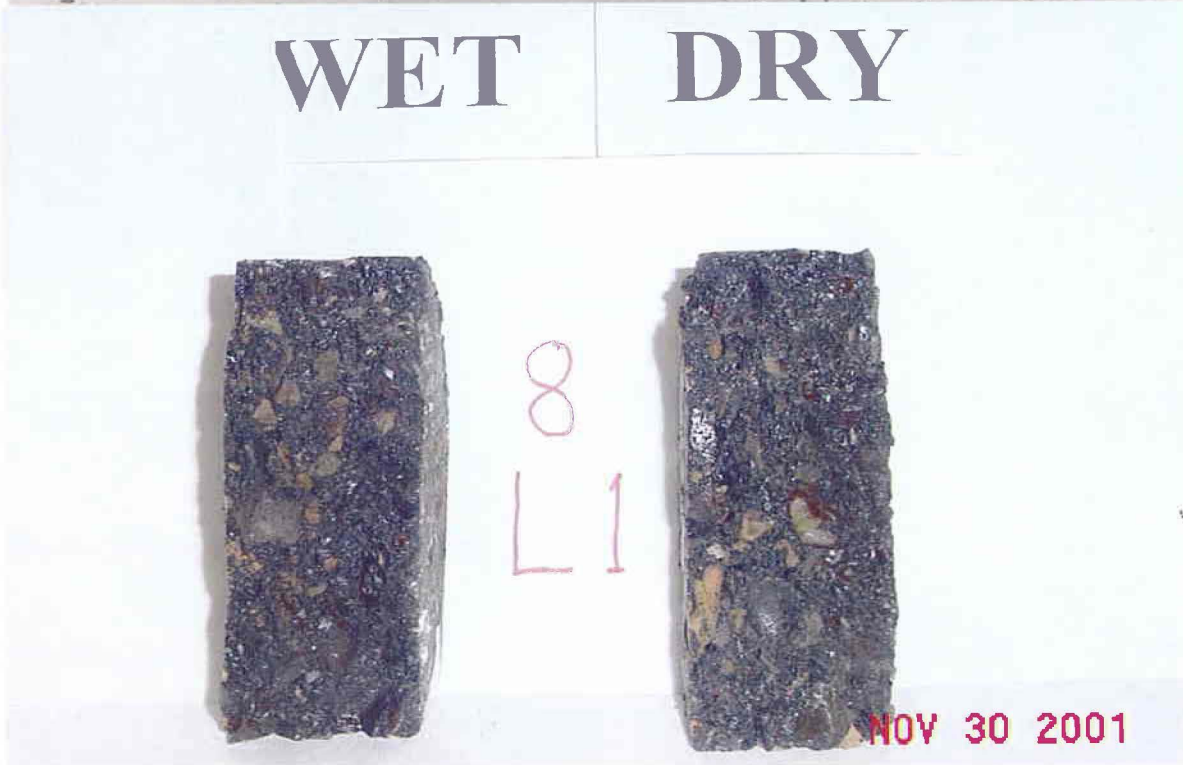
Figure B24. Photographs of the Cores after Hamburg and TSR Tests (Lufkin – Section 8 – Lp 224).
