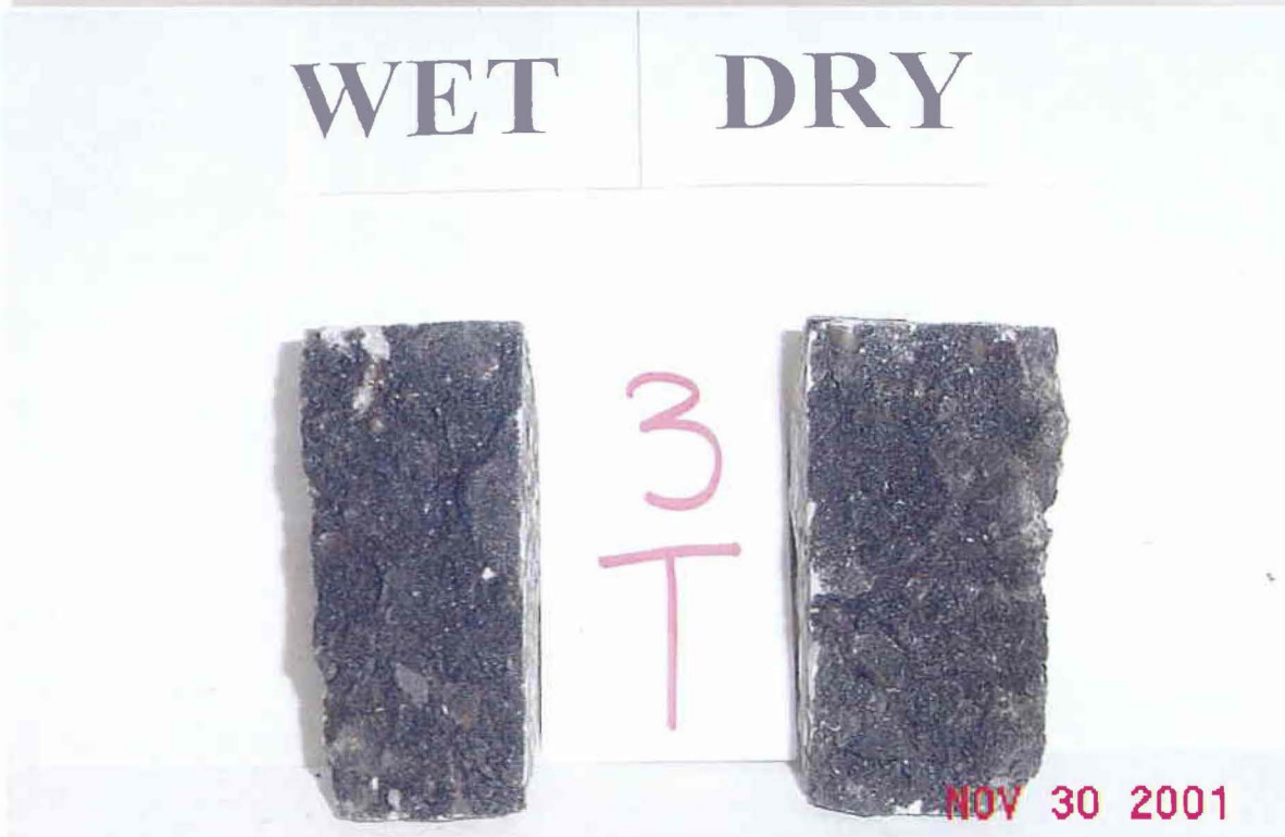
Figure B27. Photographs of the Cores after Hamburg and TSR Tests (Tyler – Section 3 – SH 31).
