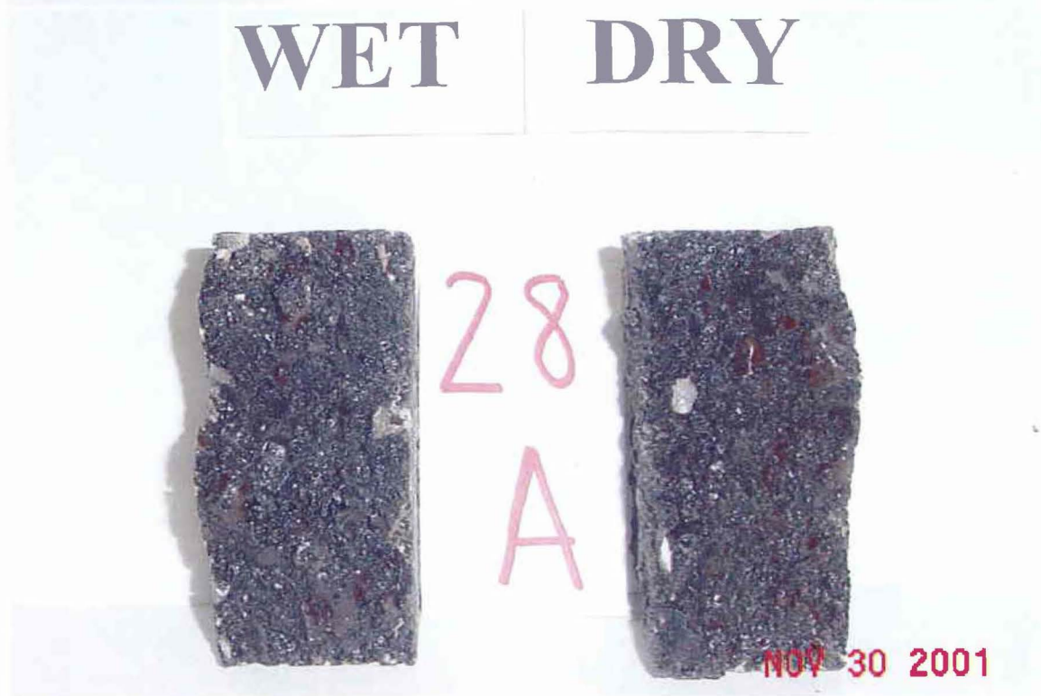
Figure B12. Photographs of the Cores after Hamburg and TSR Tests (Atlanta – Section 12 – SH 155).
