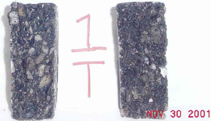
Figure B25. Photographs of the Cores after Hamburg and TSR Tests (Tyler – Section 1 – US 69).
