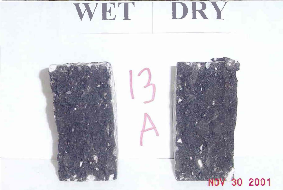
Figure B9. Photographs of the Cores after Hamburg and TSR Tests (Atlanta – Section 9 – IH 20).
