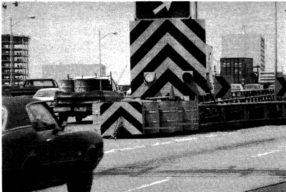
Figure 2-4. Nose Panel supplemented with Back Panel, Flashing Lights, and Chevron Alignment Signs.
