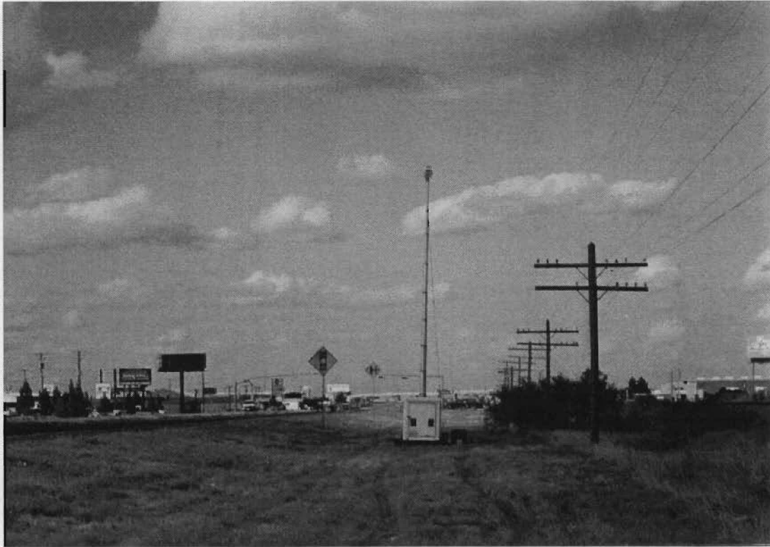
Figure 2-1. Camera Mounted on Telescoping Pole.
