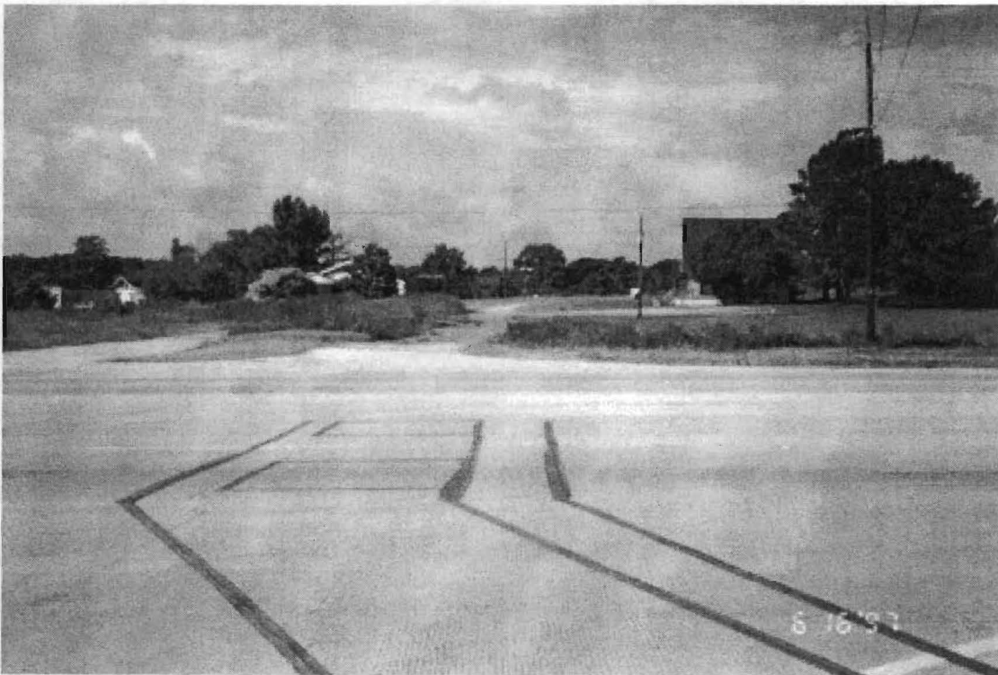
Figure 3-2. Temporary Inductive Loop and Piezoelectric Sensors.
