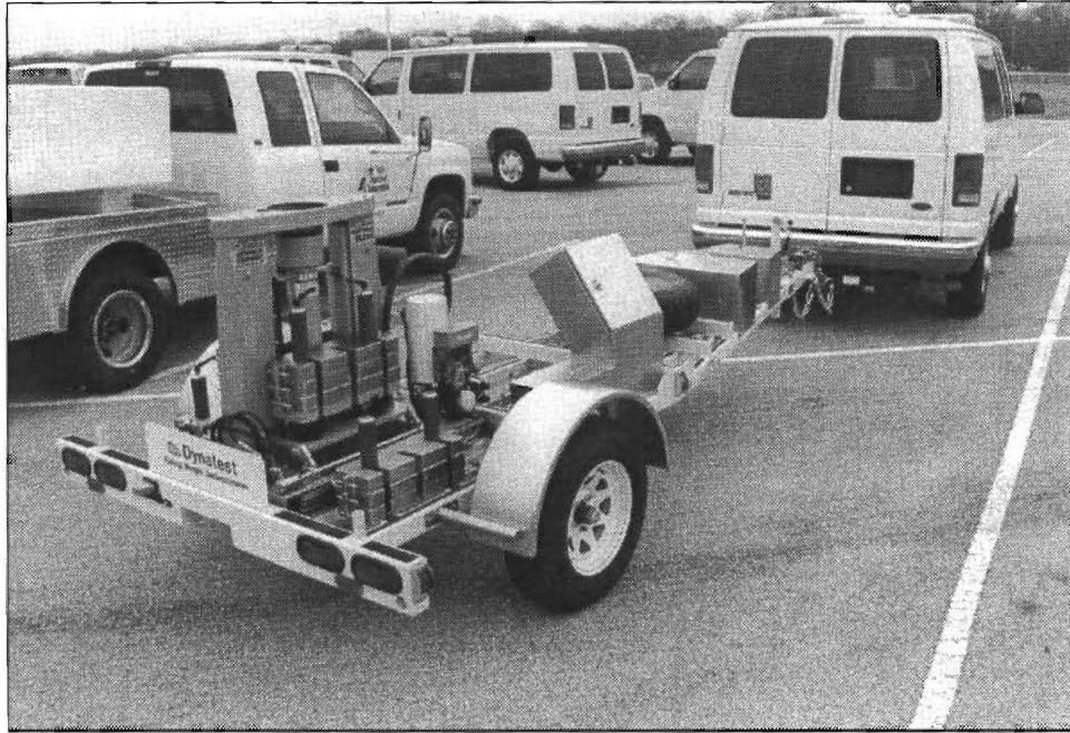
Figure 7. Illustration of the FWD
