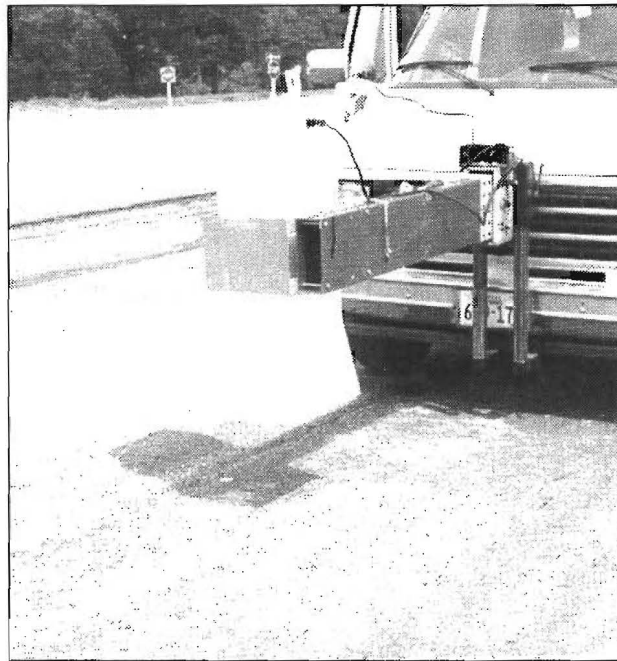
Figure 4. Front of GPR Van
