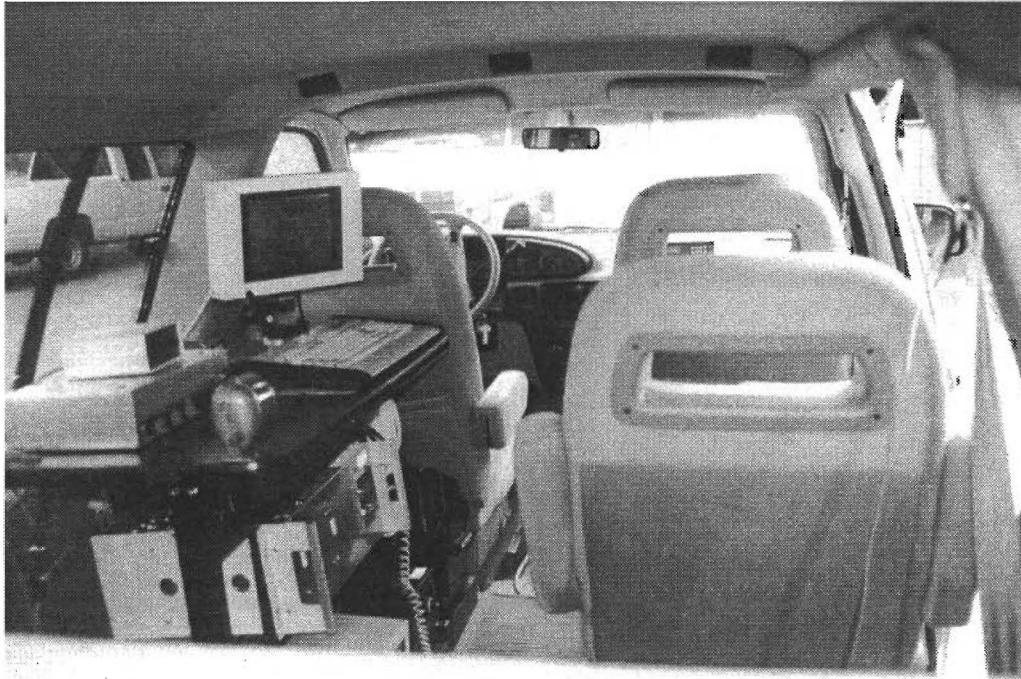
Figure 10. Example of Potential Monitor Mounting Bracket Problem
