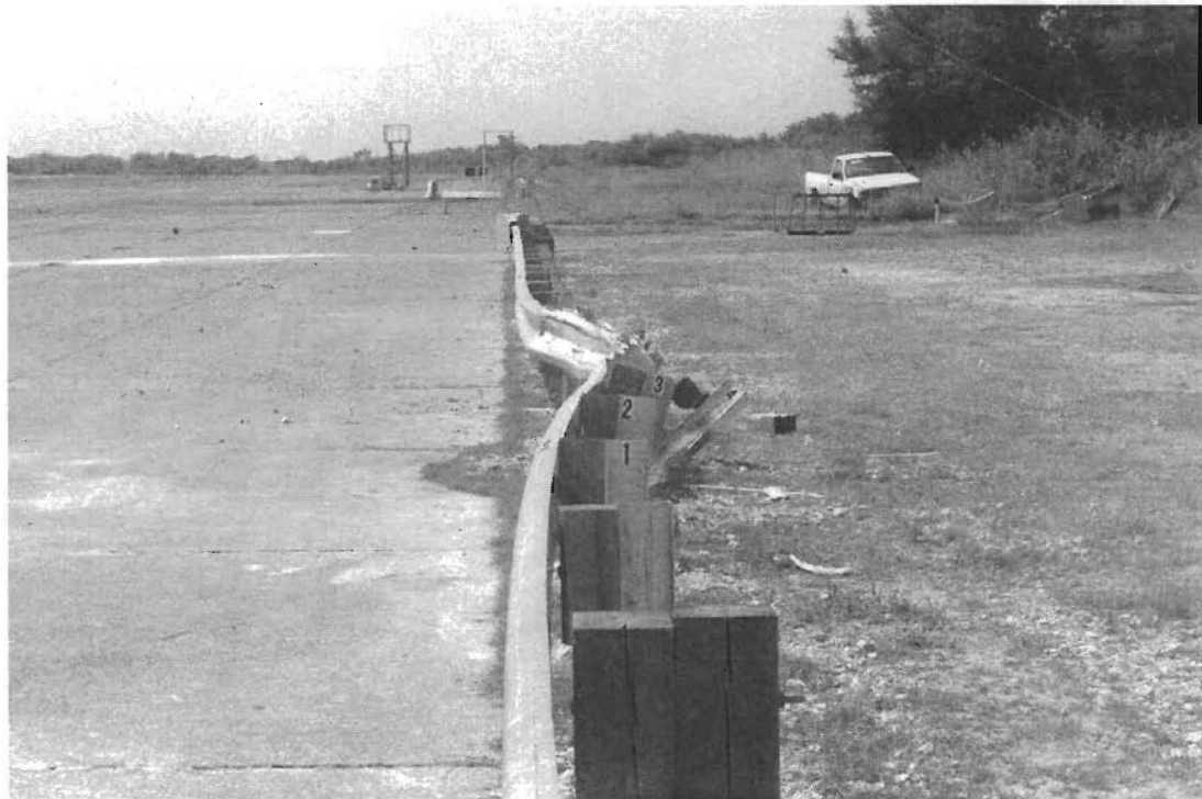
Figure 8. After impact trajectory for test 439637-1.
