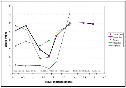
Figure 19. Site 1: SB Sp 408 to WB IH 20: Calibration Speeds (5:45–6:00 PM).
