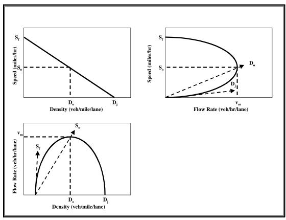
Figure 1. HCM Generalized Relationships Among Speed, Density, and Rate of Flow on Uninterrupted Flow Facilities (1).
