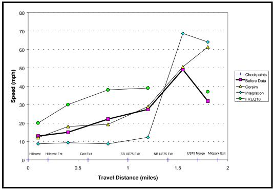
Figure 21. Site 2: EB IH 635 to NB US 75: Calibration Speeds (5:00–5:15 PM).
