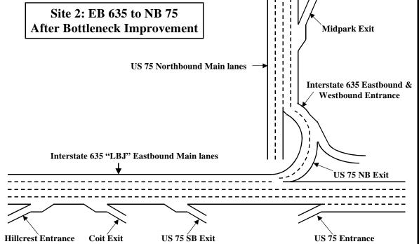
Figure 5. Site 2: EB IH 635 to NB US 75: Before and After Bottleneck Improvements.
