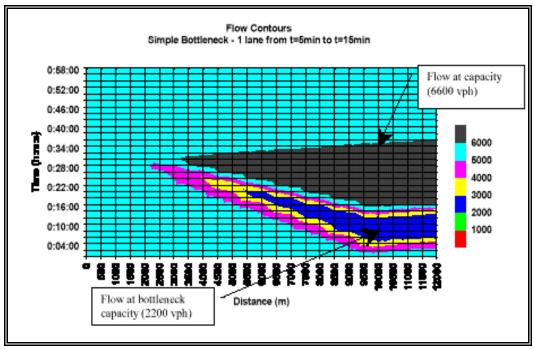
Figure 2. K-Waves 2-D Flow Contour Example (10).
