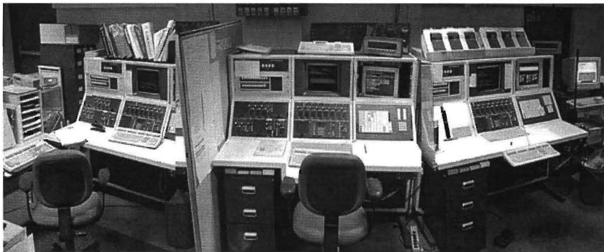
Figure A-1. Typical 911 PSAP Dispatcher Stations
