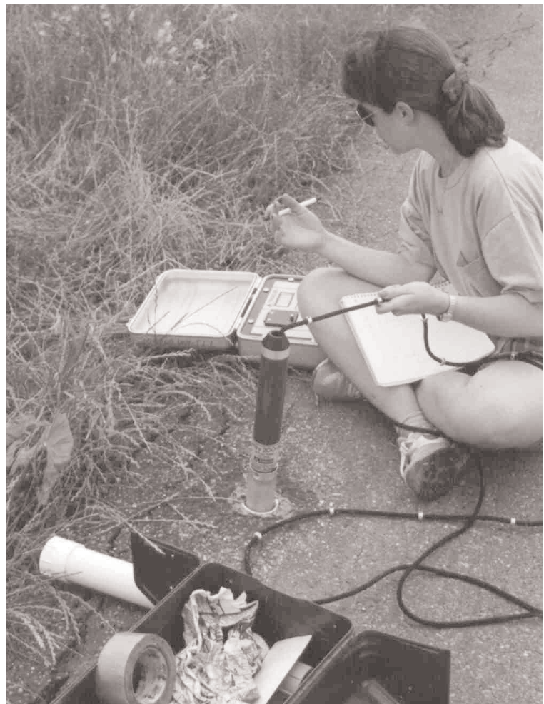
Figure 1. Probe being inserted into access tube
