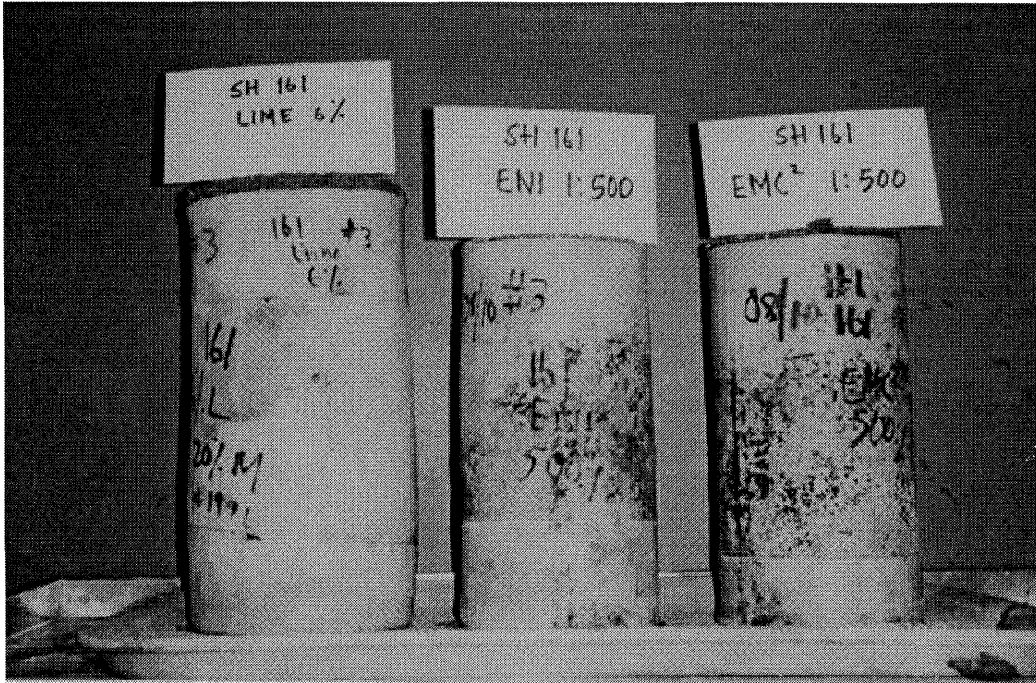
Figure 42. Photographs Showing Comparisons of Swell (Lime -6% Vs EN1-1:500, EMC 2 -1:500) - SH 161
