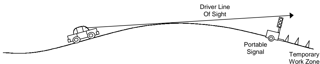
Figure 5. Driver Line of Sight Impeded by Vertical Geometry.
