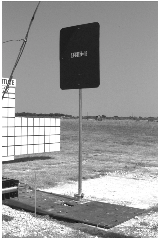
Figure 2. Typical Sign Support Installation before Pendulum Testing of Keeper Plates.
