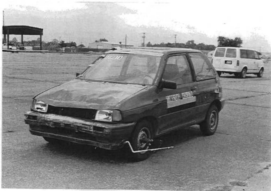
Figure 34. Vehicle After Test 439107-5.
