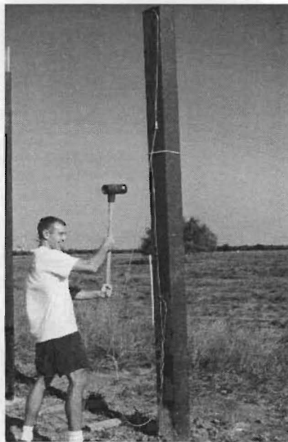
Figure 34. Impact Hammer and Column
