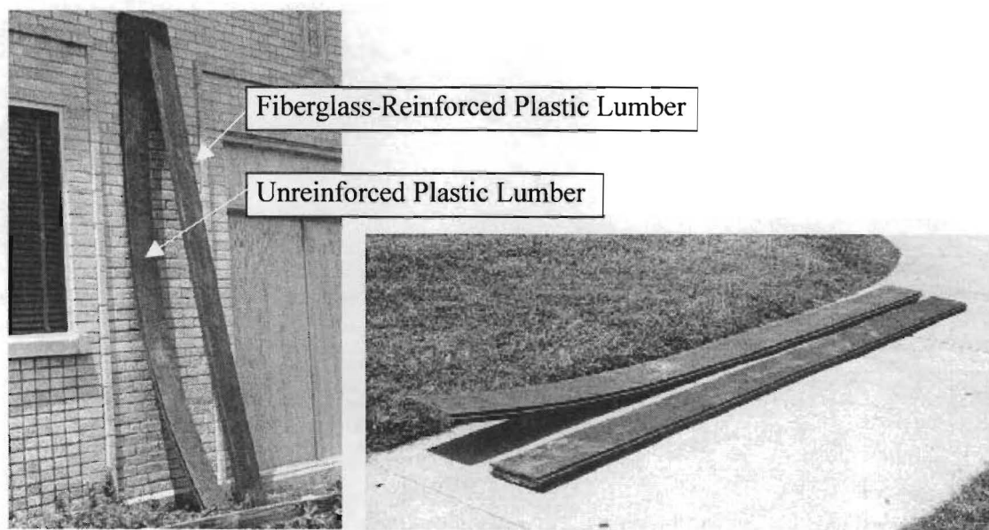
Figure 11. Sag of Fiberglass-Reinforced and Unreinforced Plastic Lumber
