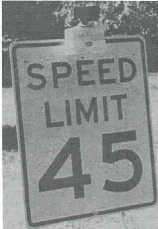
Figure 3-4. Example of a Radar Drone Mounted on a Speed Limit Sign
