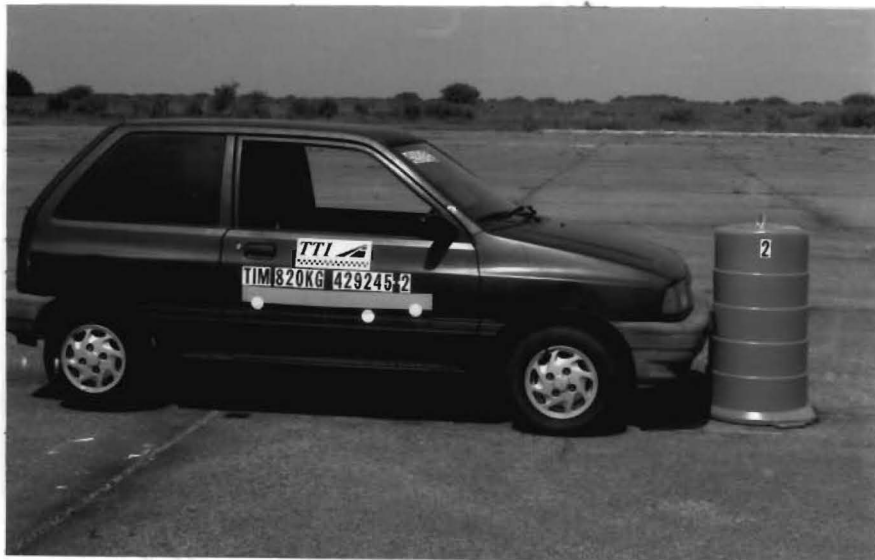
Figure 1. Photographs of Typical Setup for Full-Scale Crash Tests
