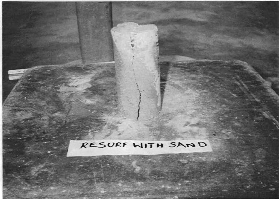
Fig. 2.9. A Tested Slanting Shear Specimen of Resurf Blended with Sand as Repair Material.
