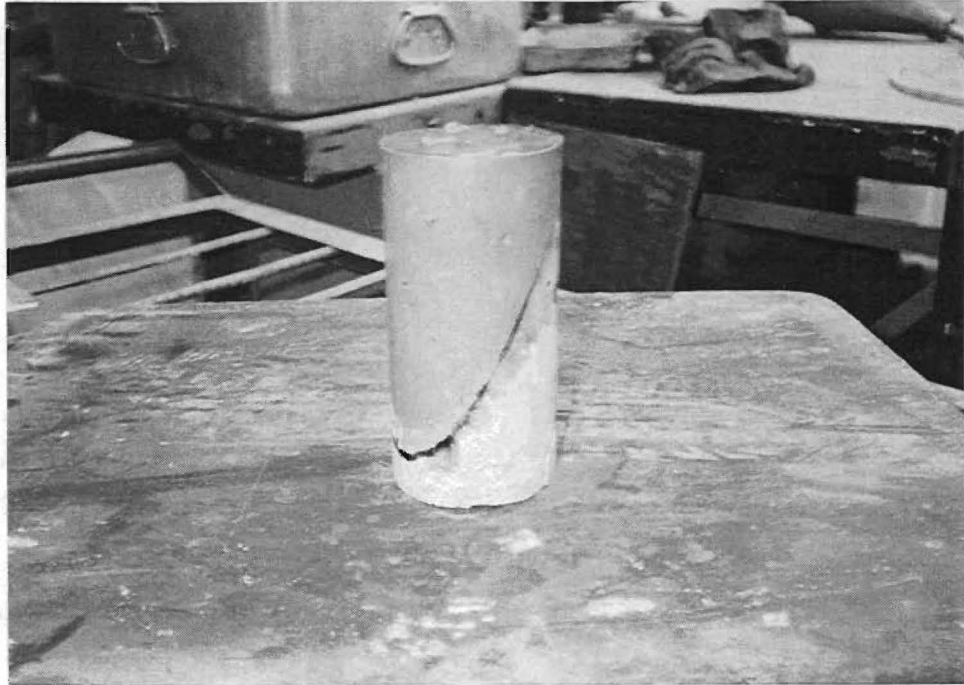
Fig. 2.10. A Finished Slanting Shear Specimen of Sylcrete Mender Blended with Aggregates.
