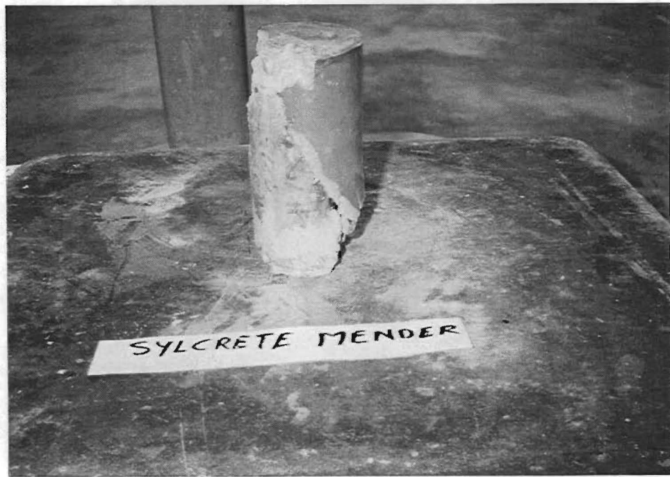
Fig. 2.11. A tested slanting shear specimen of Sylcrete mender blended with aggregates.
