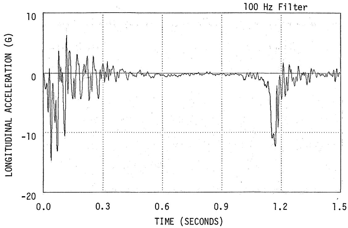
Figure B-78. Vehicle Longitudinal Acceleration, Test 9-1.
