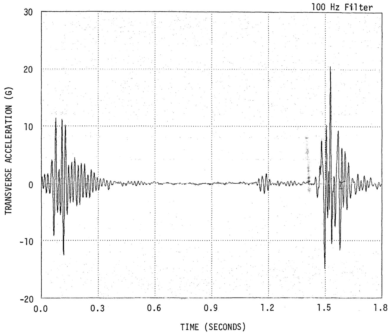
Figure B-35. Vehicle Transverse Acceleration, Test 5-1.
