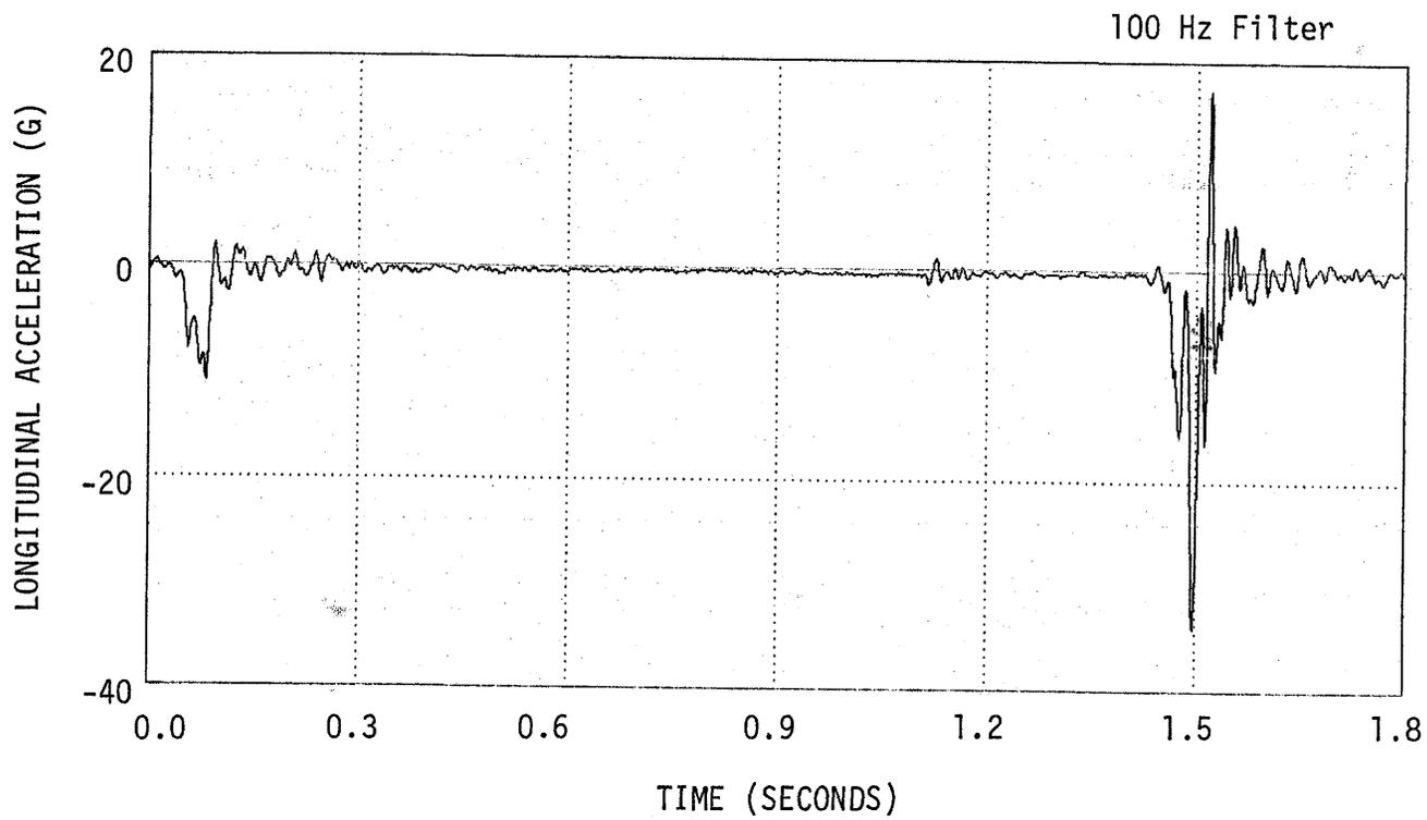
Figure B-36. Vehicle Longitudinal Acceleration, Test 5-1.
