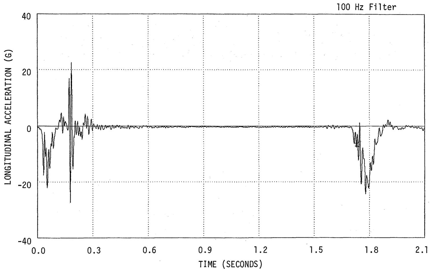
Figure B-26. Vehicle Longitudinal Acceleration, Test 1-4.
