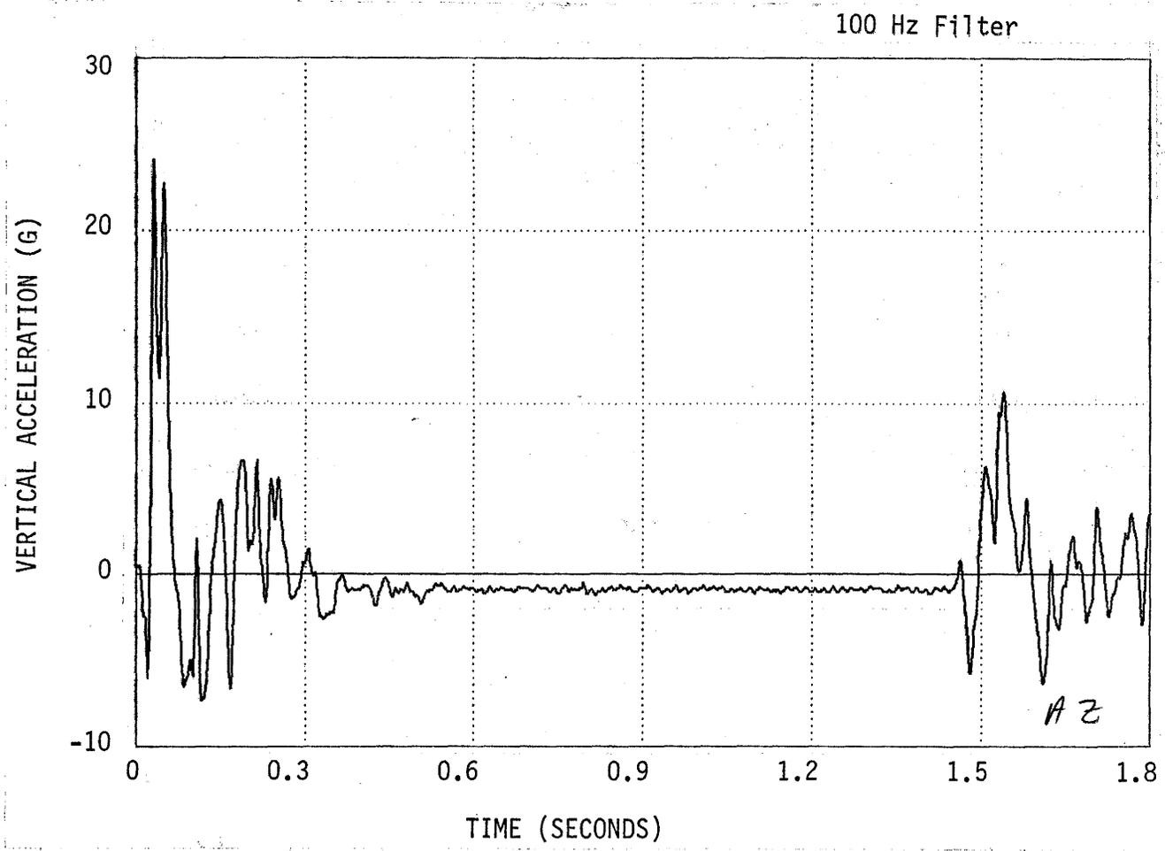
Figure B-22. Vehicle Vertical Acceleration, Test 1-3.
