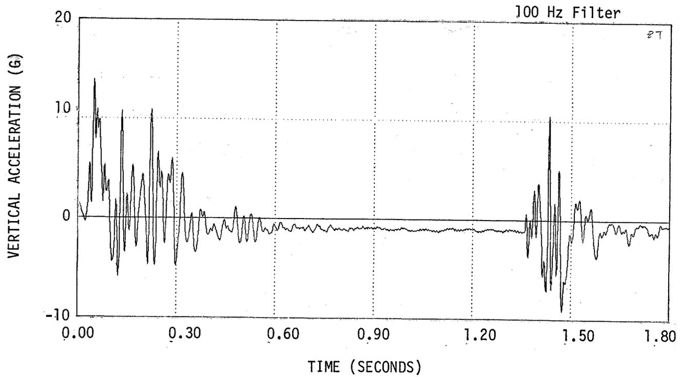
Figure B-65. Vehicle Vertical Acceleration, Test 7-5.
