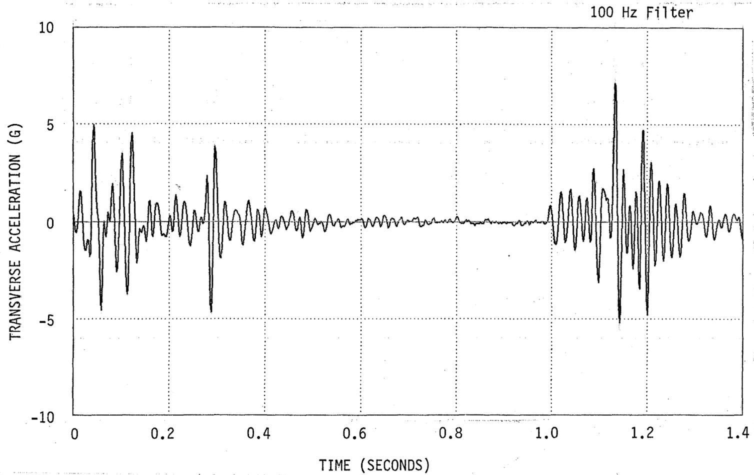
Figure B-6. Vehicle Transverse Acceleration, Test 1-1.
