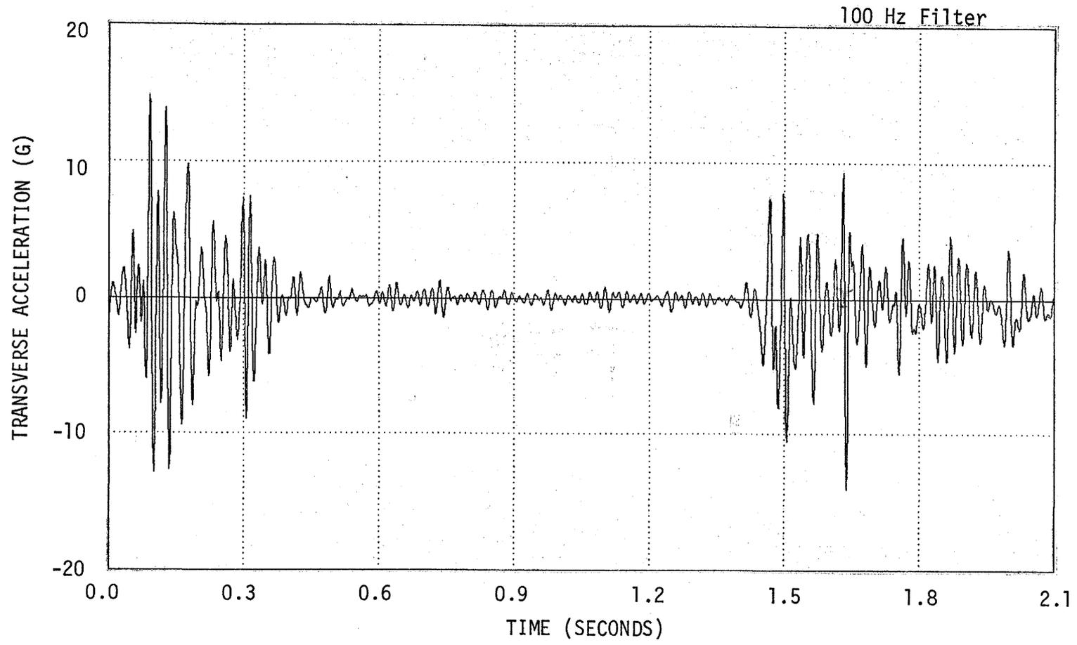
Figure B-70. Vehicle Transverse Acceleration, Test 7-6.
