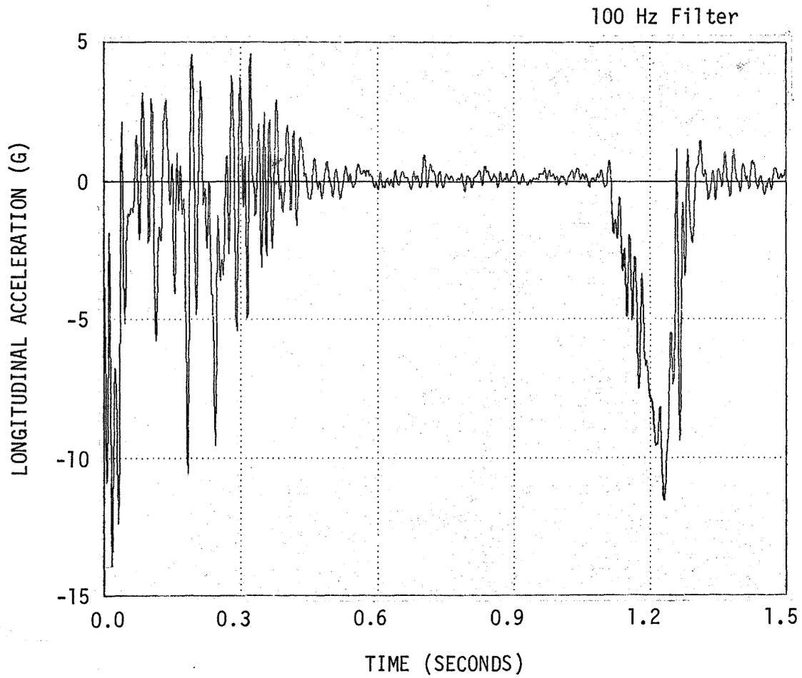
Figure B-41. Vehicle Longitudinal Acceleration, Test 7-1.
