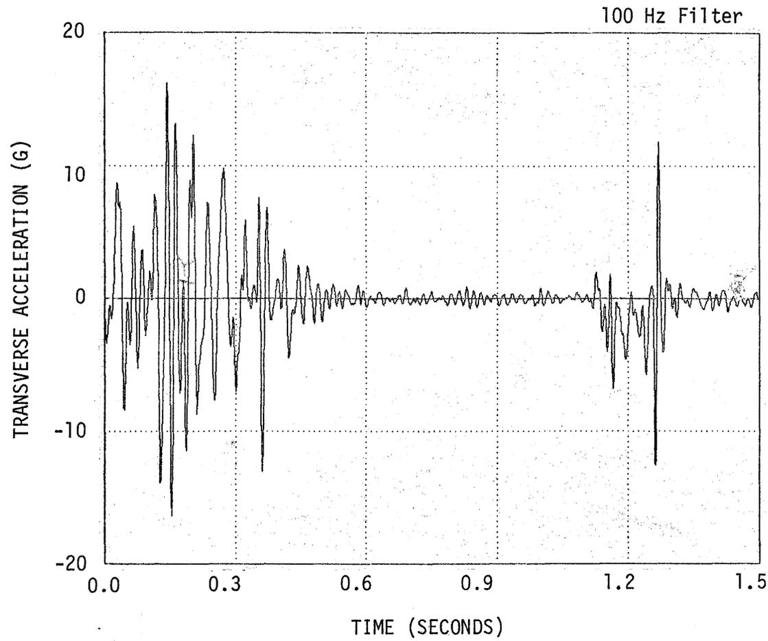
Figure B-42. Vehicle Transverse Acceleration, Test 7-1.
