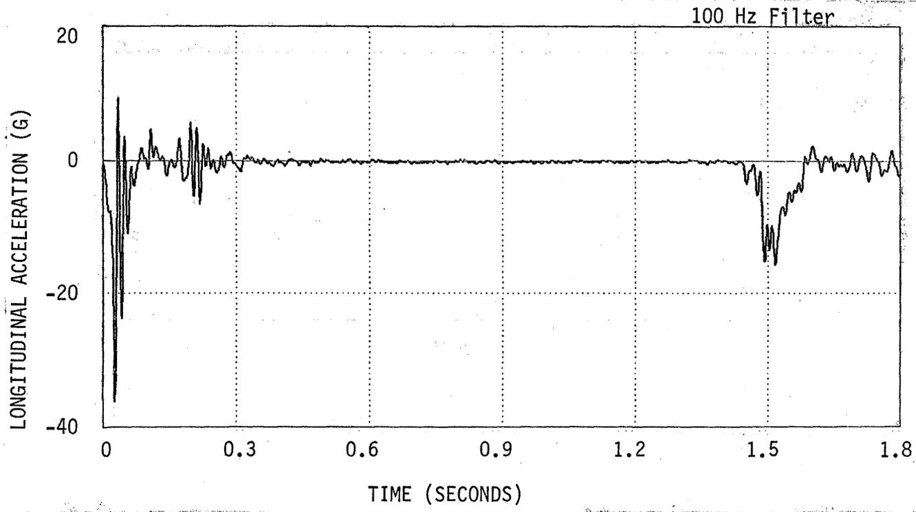
Figure B-20. Vehicle Longitudinal Acceleration, Test 1-3.
