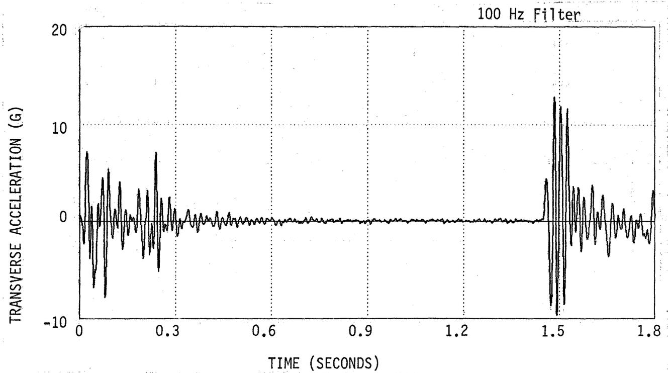
Figure B-21. Vehicle Transverse Acceleration, Test 1-3.
