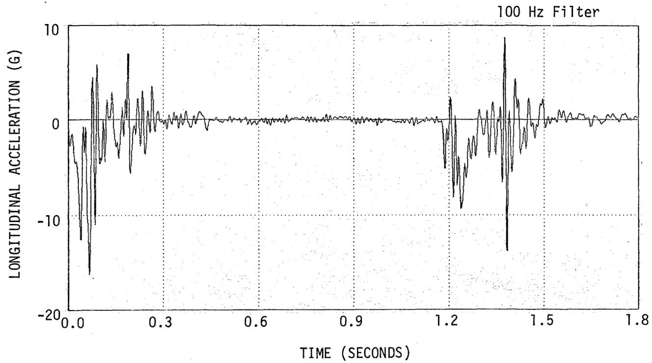
Figure B-85. Vehicle Longitudinal Acceleration, Test 9-2.
