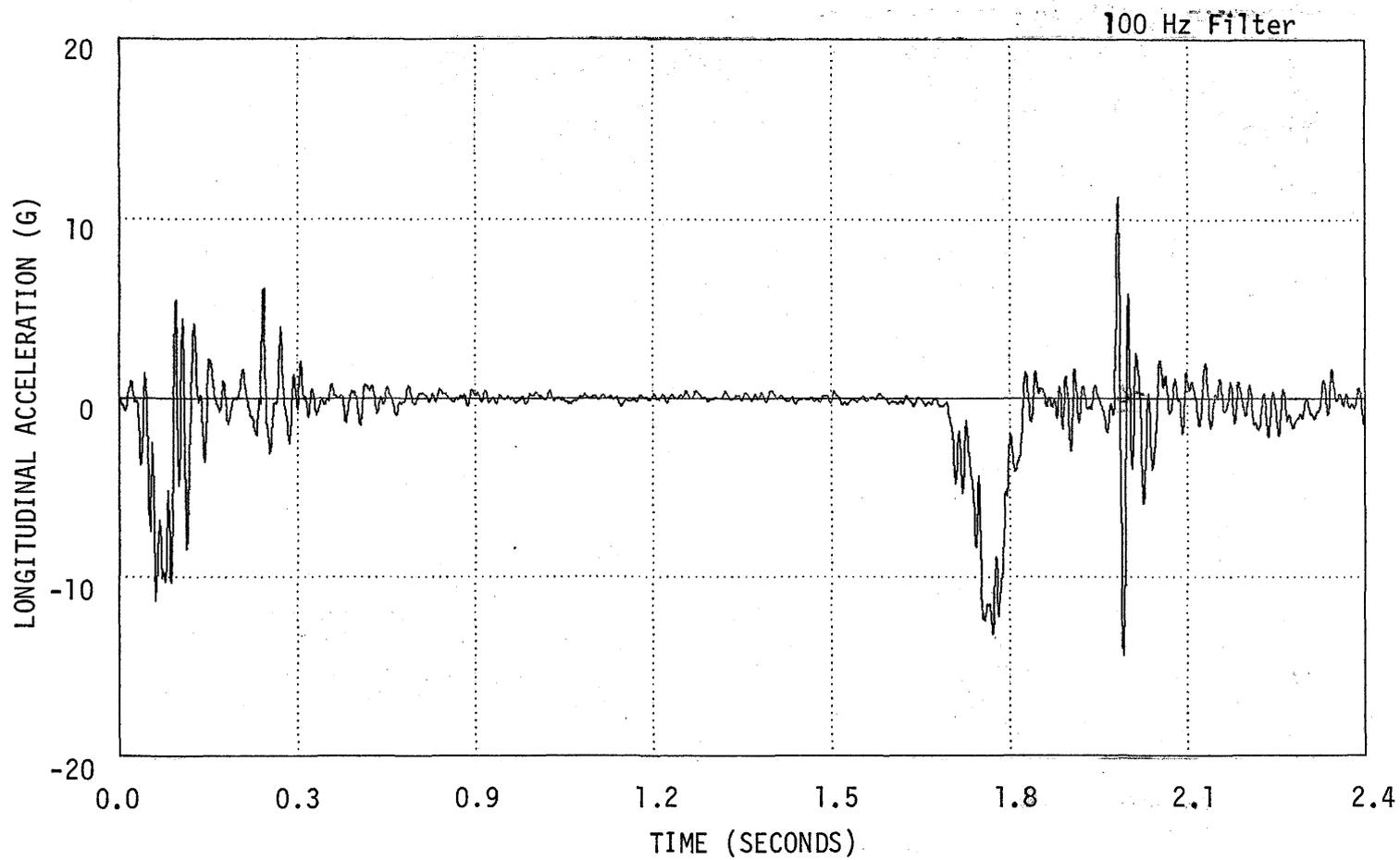
Figure B-69. Vehicle Longitudinal Acceleration, Test 7-6.
