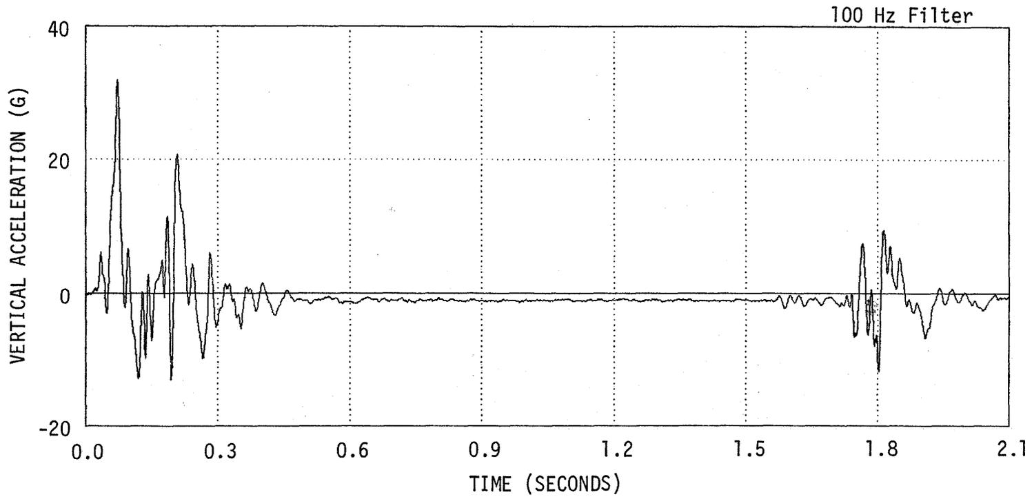
Figure B-28. Vehicle Vertical Acceleration, Test 1-4.
