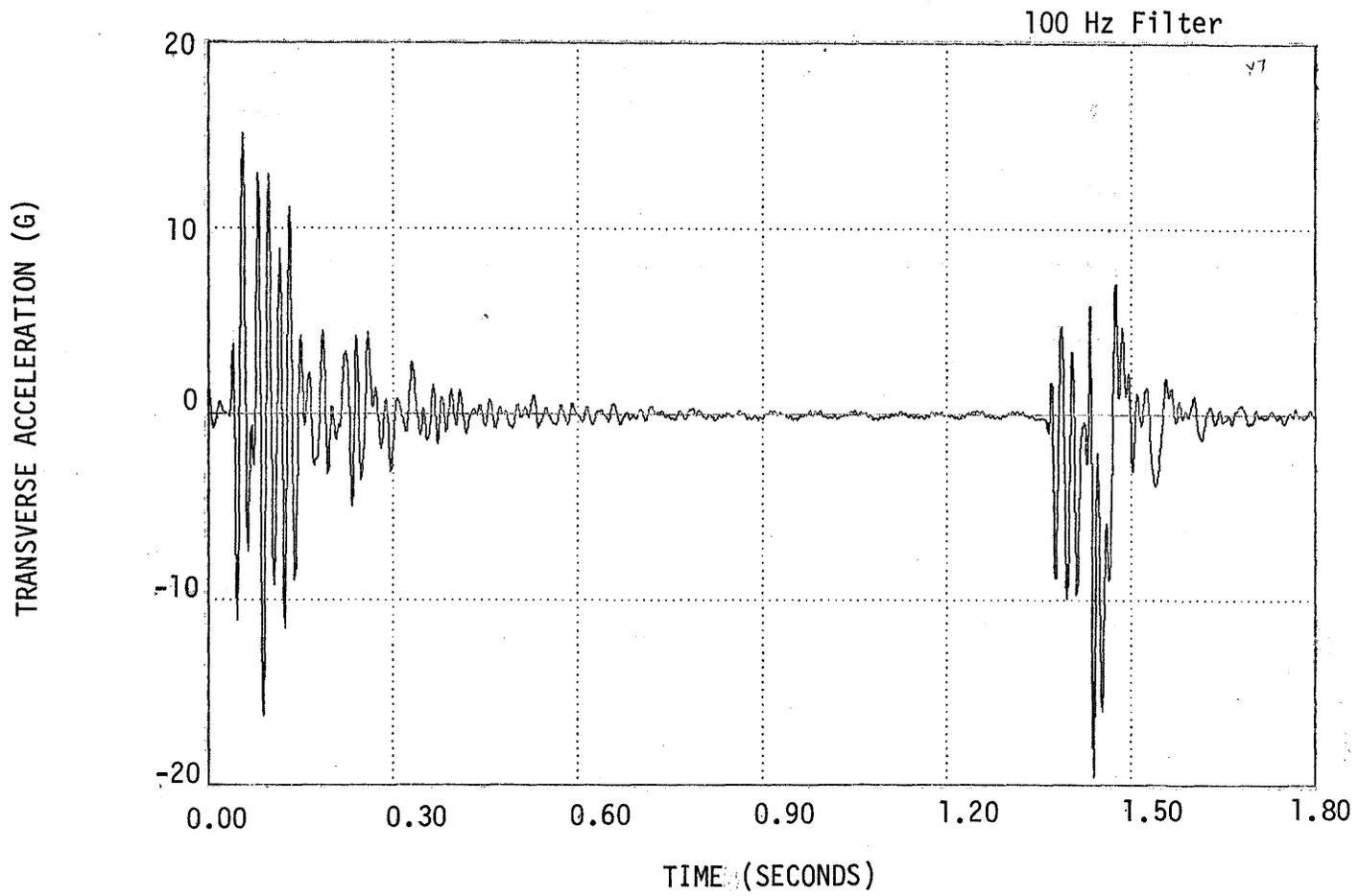
Figure B-64. Vehicle Transverse Acceleration, Test 7-5.
