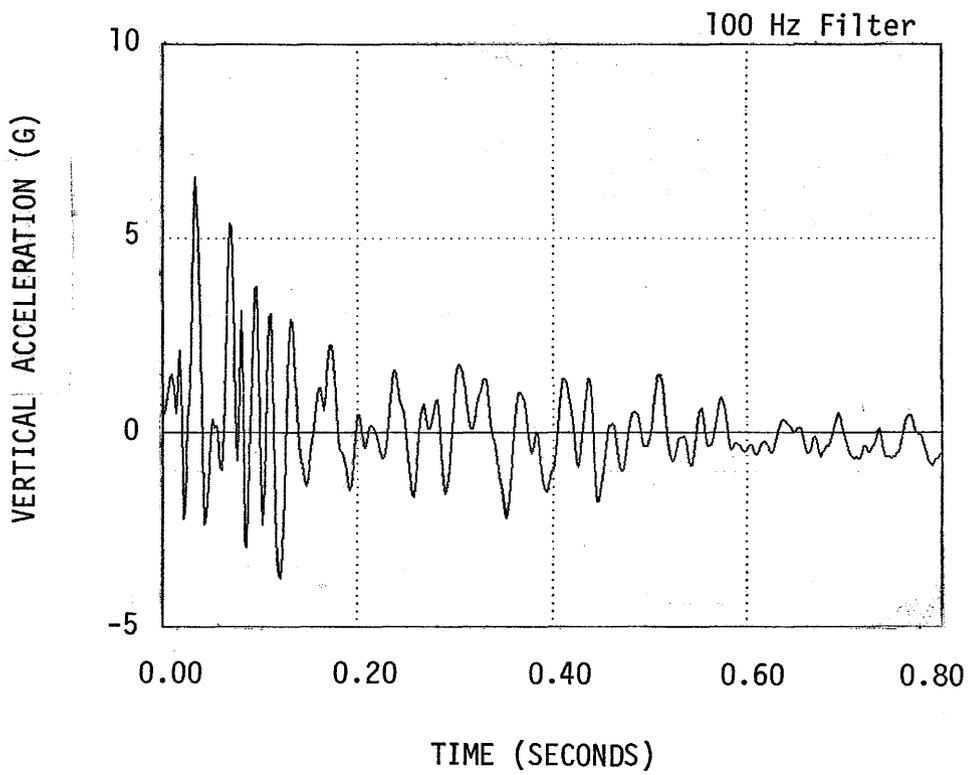
Figure B-57. Vehicle Vertical Acceleration, Test 7-4.
