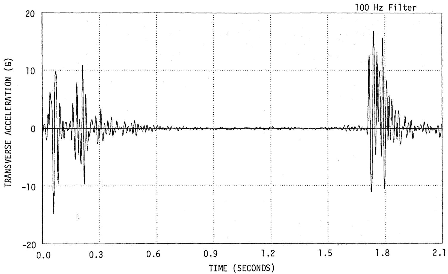
Figure B-27. Vehicle Transverse Acceleration, Test 1-4.
