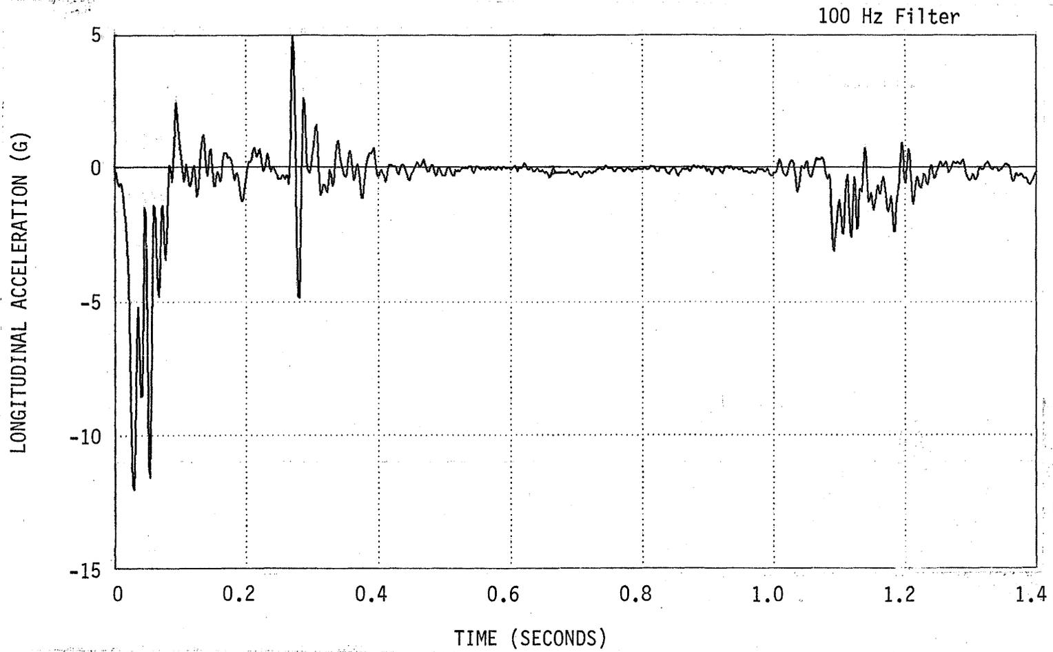
Figure B-5. Vehicle Longitudinal Acceleration, Test 1-1.
