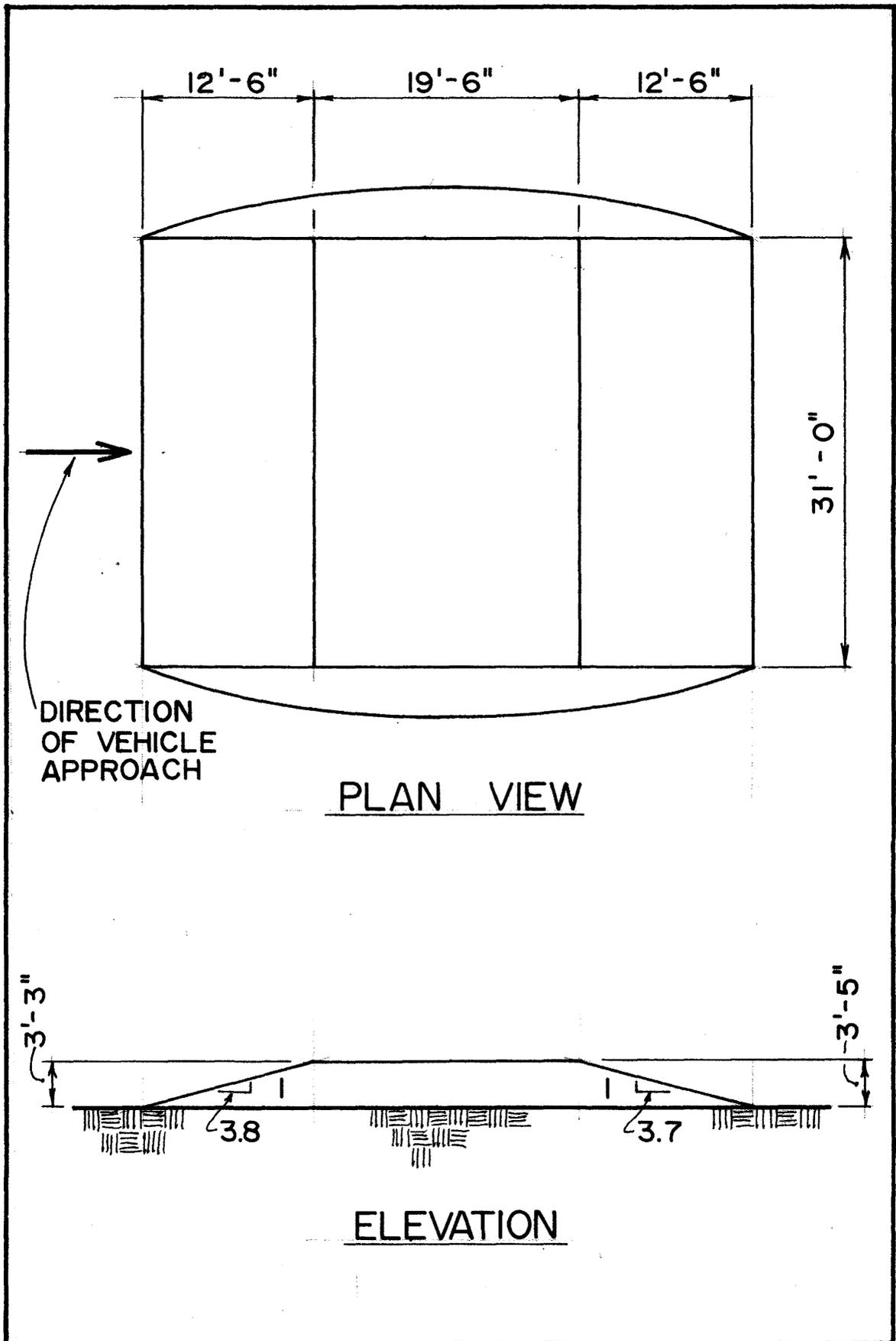
Figure 2. Berm Dimensions for Tests 1-1 through 1-4.
