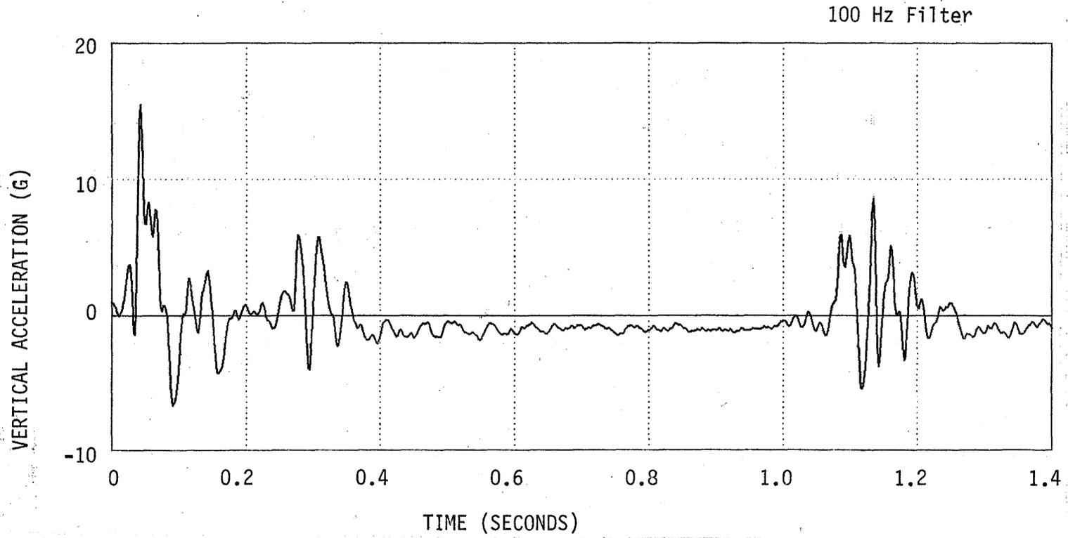
Figure B-7. Vehicle Vertical Acceleration, Test 1-1.
