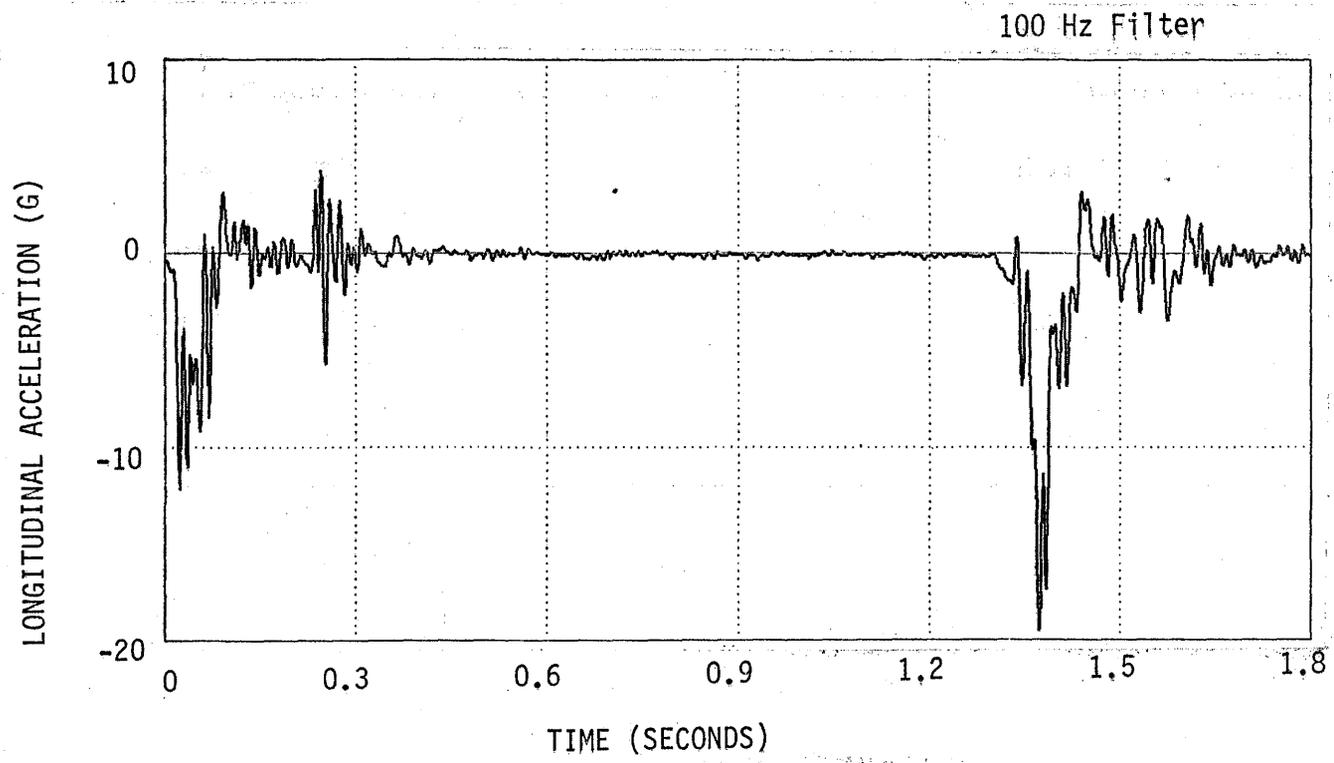
Figure B-12. Vehicle Longitudinal Acceleration, Test 1-2.
