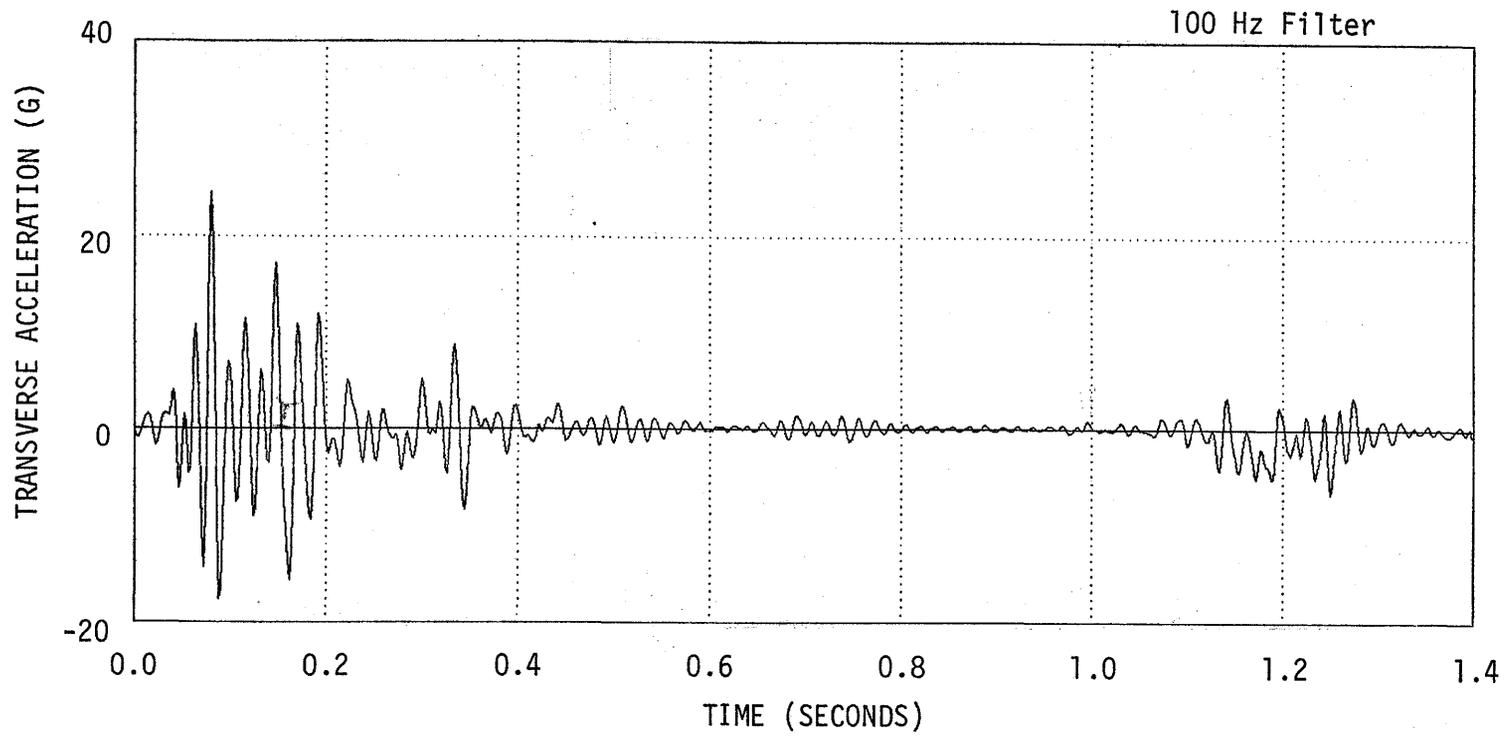
Figure B-49. Vehicle Transverse Acceleration, Test 7-2.
