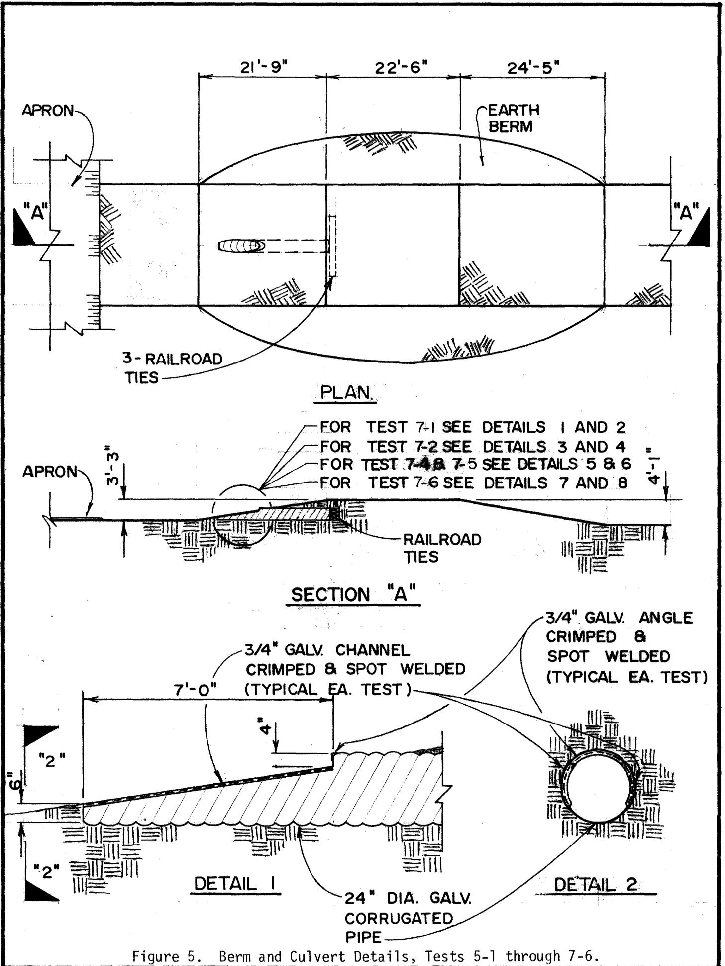
Figure 5. Berm and Culvert Details, Tests 5-1 through 7-6.
