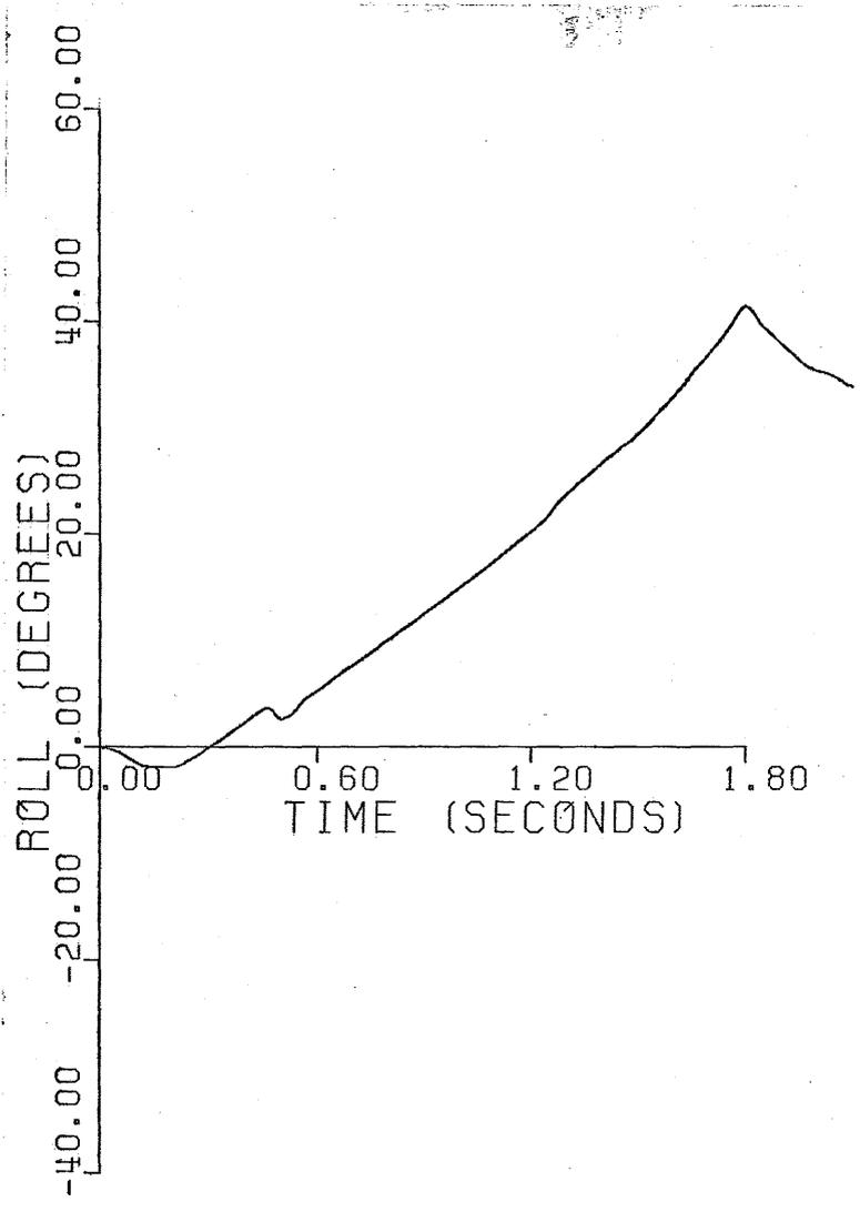
Figure B-29. Vehicle Roll, Test 1-4.
