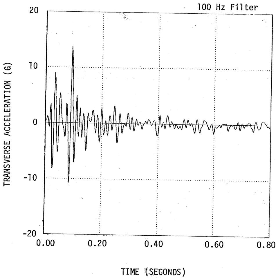
Figure B-56. Vehicle Transverse Acceleration, Test 7-4.
