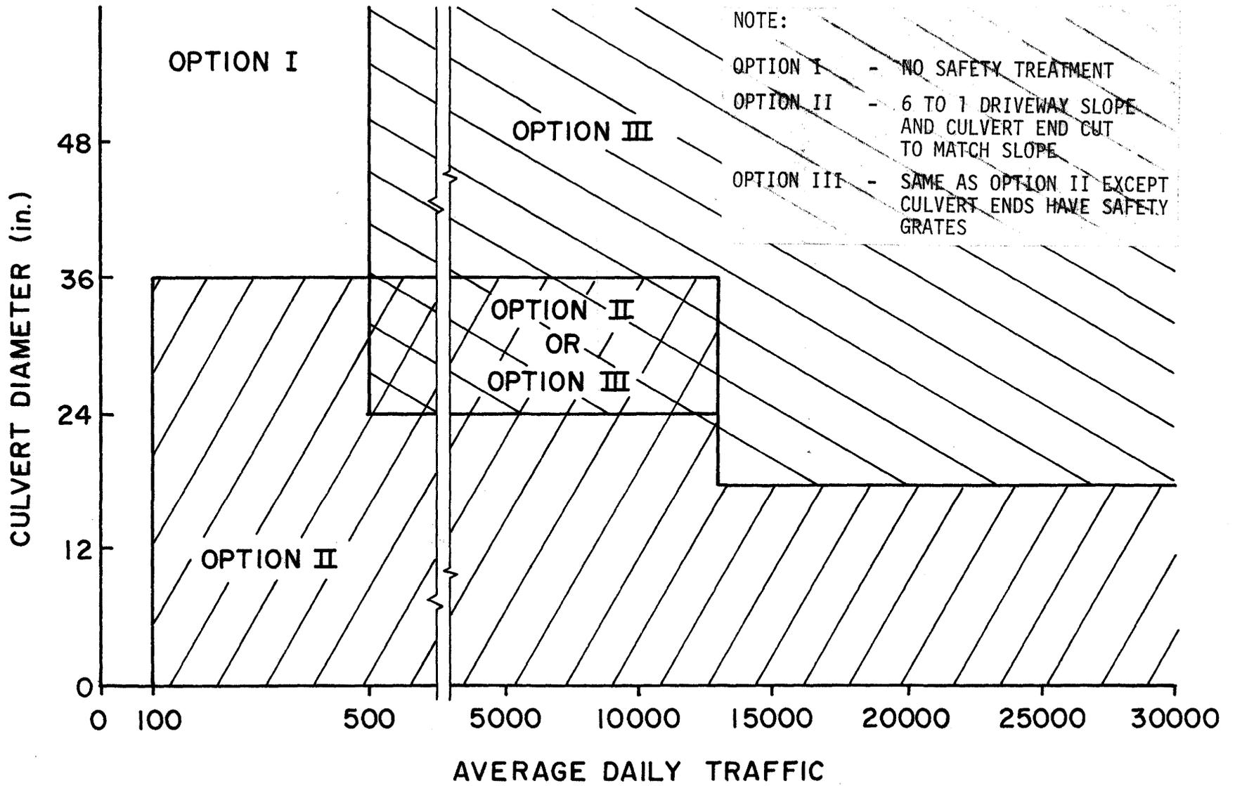
FIGURE 19. WARRANTS FOR SAFETY TREATMENT OF PARALLEL DRAINAGE CULVERTS
