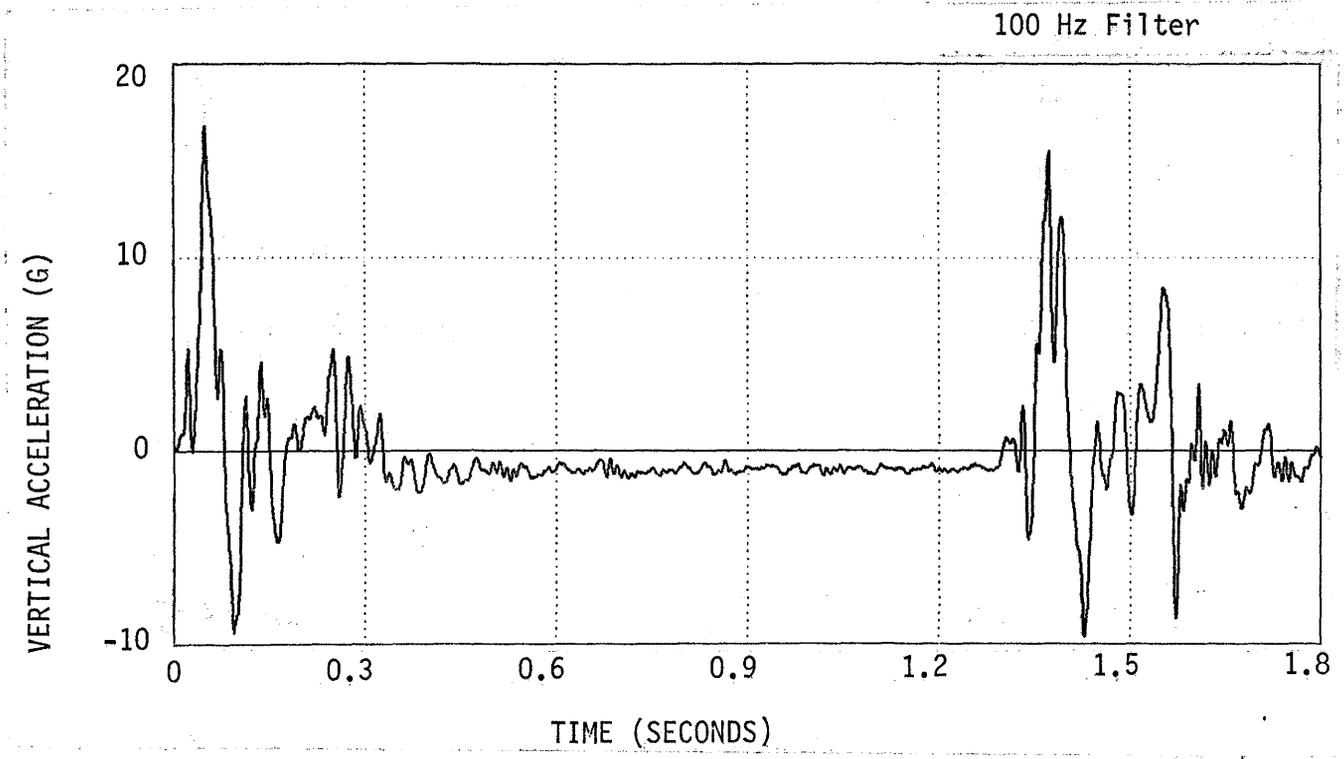
Figure B-14. Vehicle Vertical Acceleration, Test 1-2.
