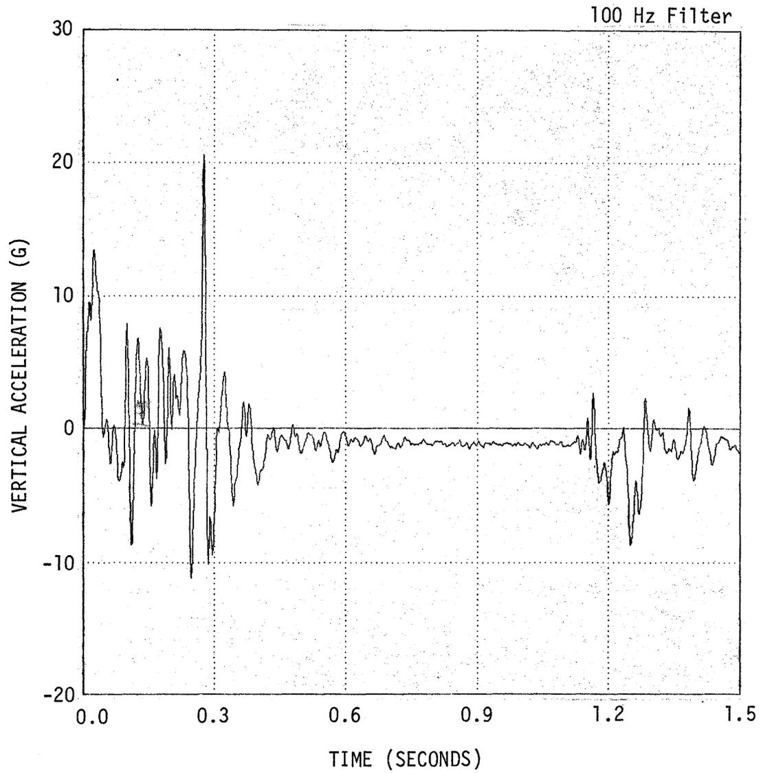
Figure B-43. Vehicle Vertical Acceleration, Test 7-1.
