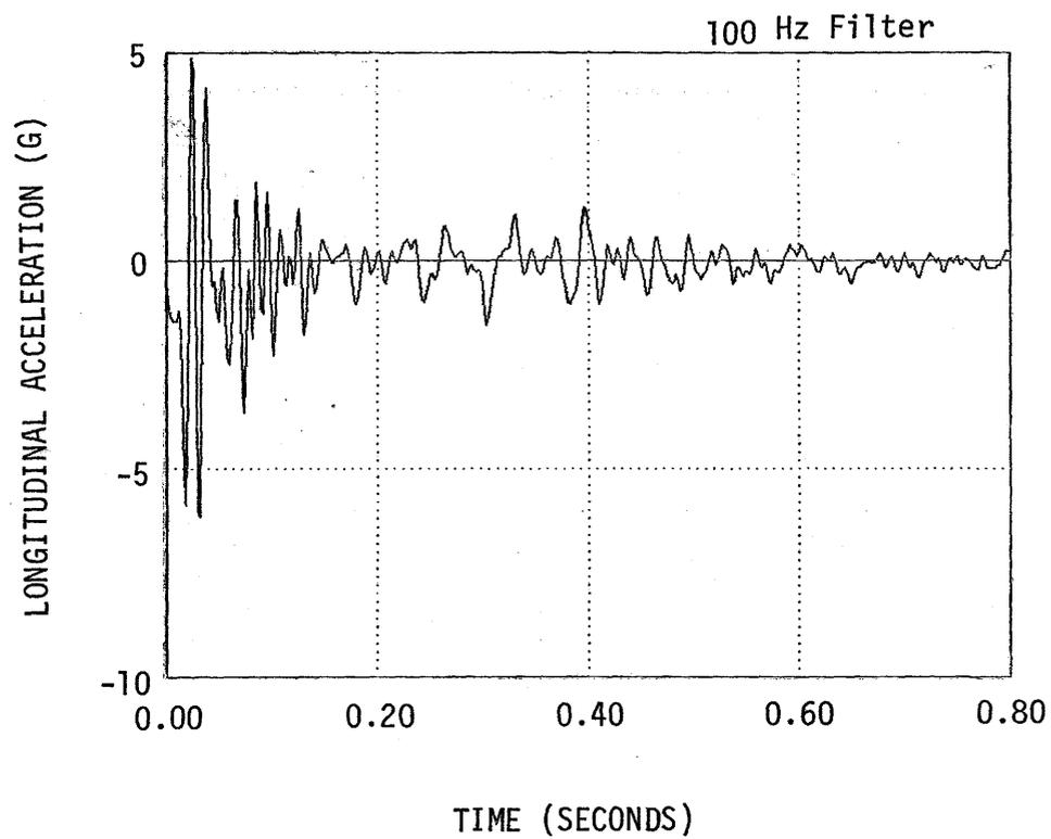
Figure B-55. Vehicle Longitudinal Acceleration, Test 7-4.
