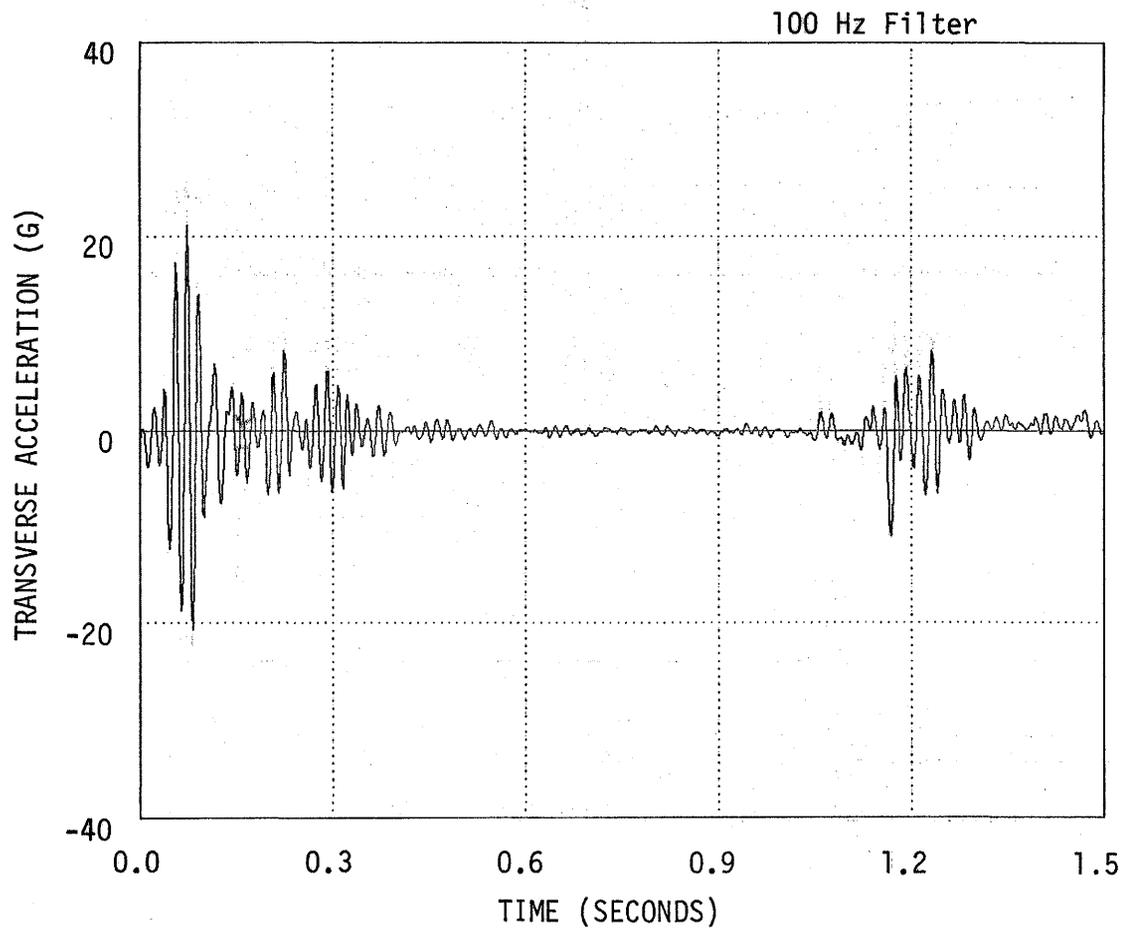
Figure B-79. Vehicle Transverse Acceleration, Test 9-1.
