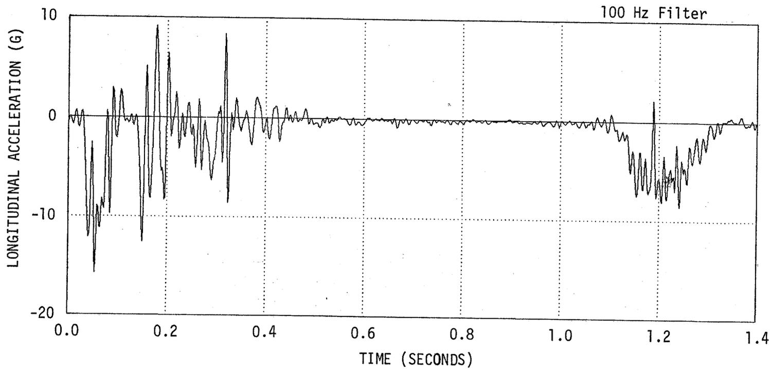
Figure B-48. Vehicle Longitudinal Acceleration, Test 7-2.
