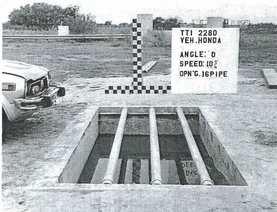
b) Grated Culvert Setup
